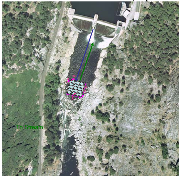
Figure 1c. Plan view of chiller location on Poe Reach; Pipe size = 4 ft; flow rate = 200 cfs
