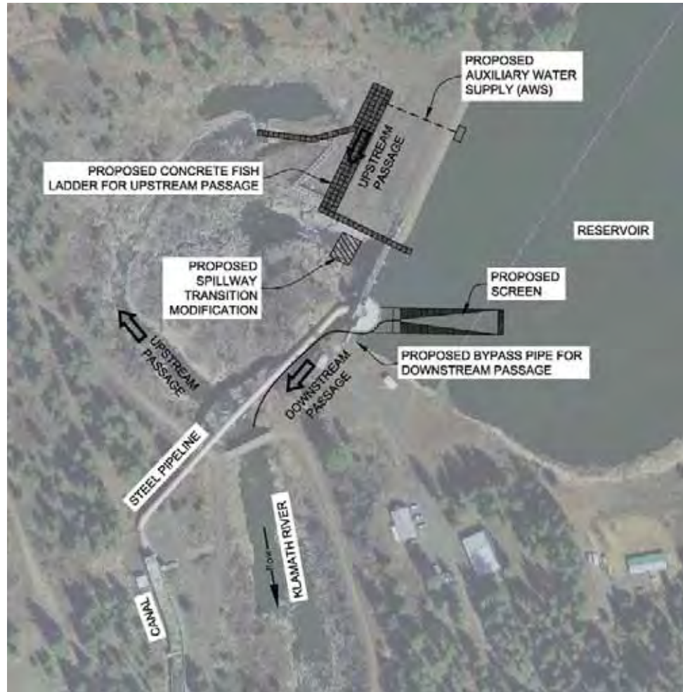
Figure 2-23. Conceptual Layout of J.C. Boyle Fish Passage Facilities.
