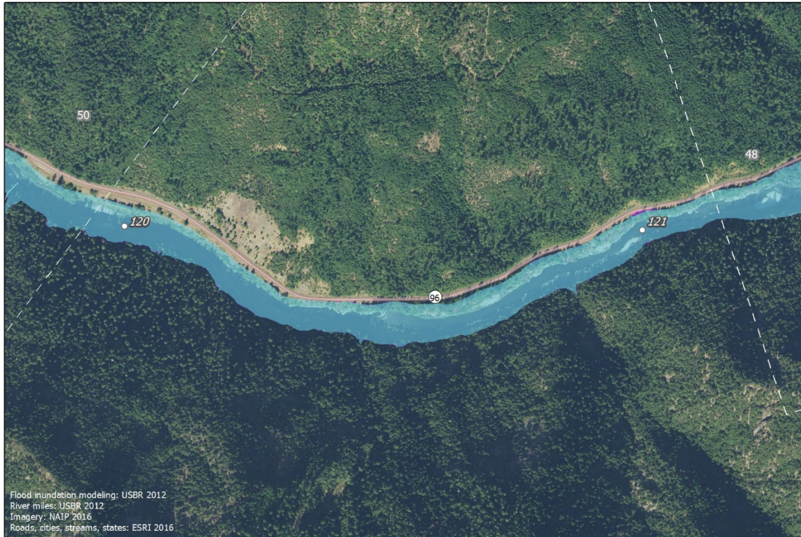
Modeled 100-year Flood Inundation Extent No Project (USBR) Proposed Project (USBR) River miles 0 200 400 Feet Map 49 of 57 Stillwater Sciences Klamath River
