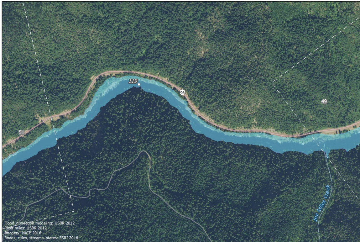
Modeled 100-year Flood Inundation Extent No Project (USBR) Proposed Project (USBR) River miles 0 200 400 Feet Map 50 of 57 Stillwater Sciences Klamath River
