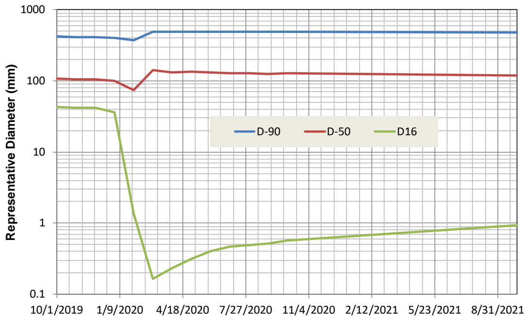
Figure F1-28. Simulated Bed Substrate Size from Iron Gate Dam to Bogus Creek Following Dam Removal. Based on simulation results provided by Reclamation, March 2012.
