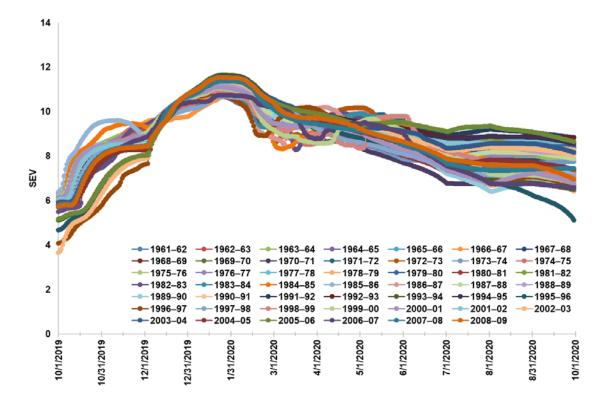
Figure E-1. Example SEV Values Assuming a 30-day Exposure at Iron Gate Dam, based on the SSC Predictions using the SRH-1D Model.
