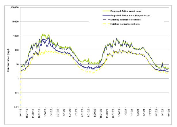
Figure E-3. Comparison of SSC at Klamath Station (RM 5) under Existing Conditions and the Proposed Project, as Predicted Using SRH-1D Model.
