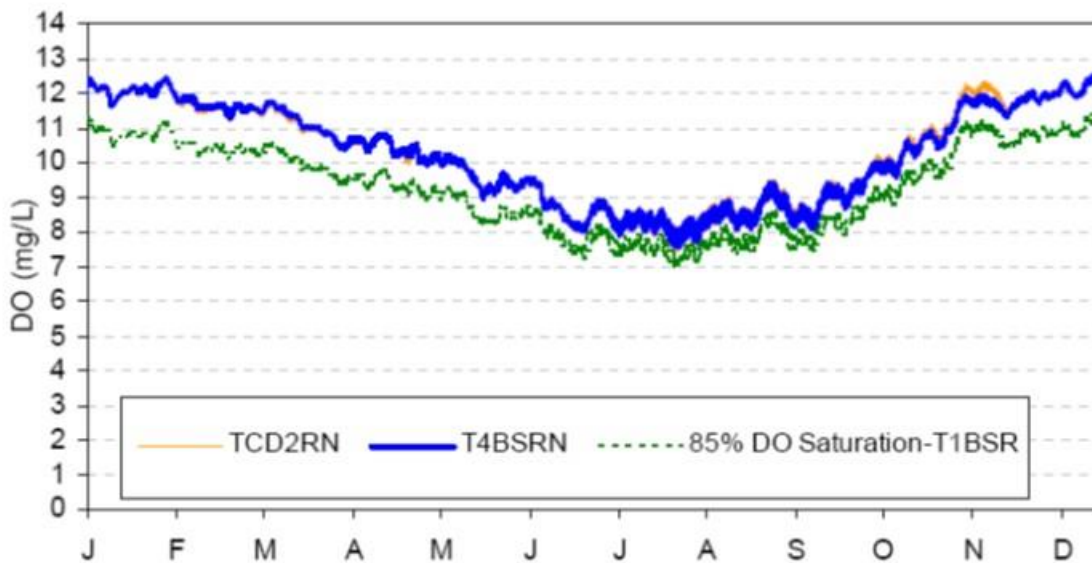
Figure 3.2-23. Predicted Dissolved Oxygen Just Upstream of the Confluence with the Trinity River (RM 43.3) for the Klamath River TMDL Scenarios Similar to the Proposed Project (“TMDL dams-out, Oregon” [TOD2RN] Scenario) and Existing Conditions (“TMDL dams-in” [T4BSRN] Scenario). Source: North Coast Regional Board 2010.
