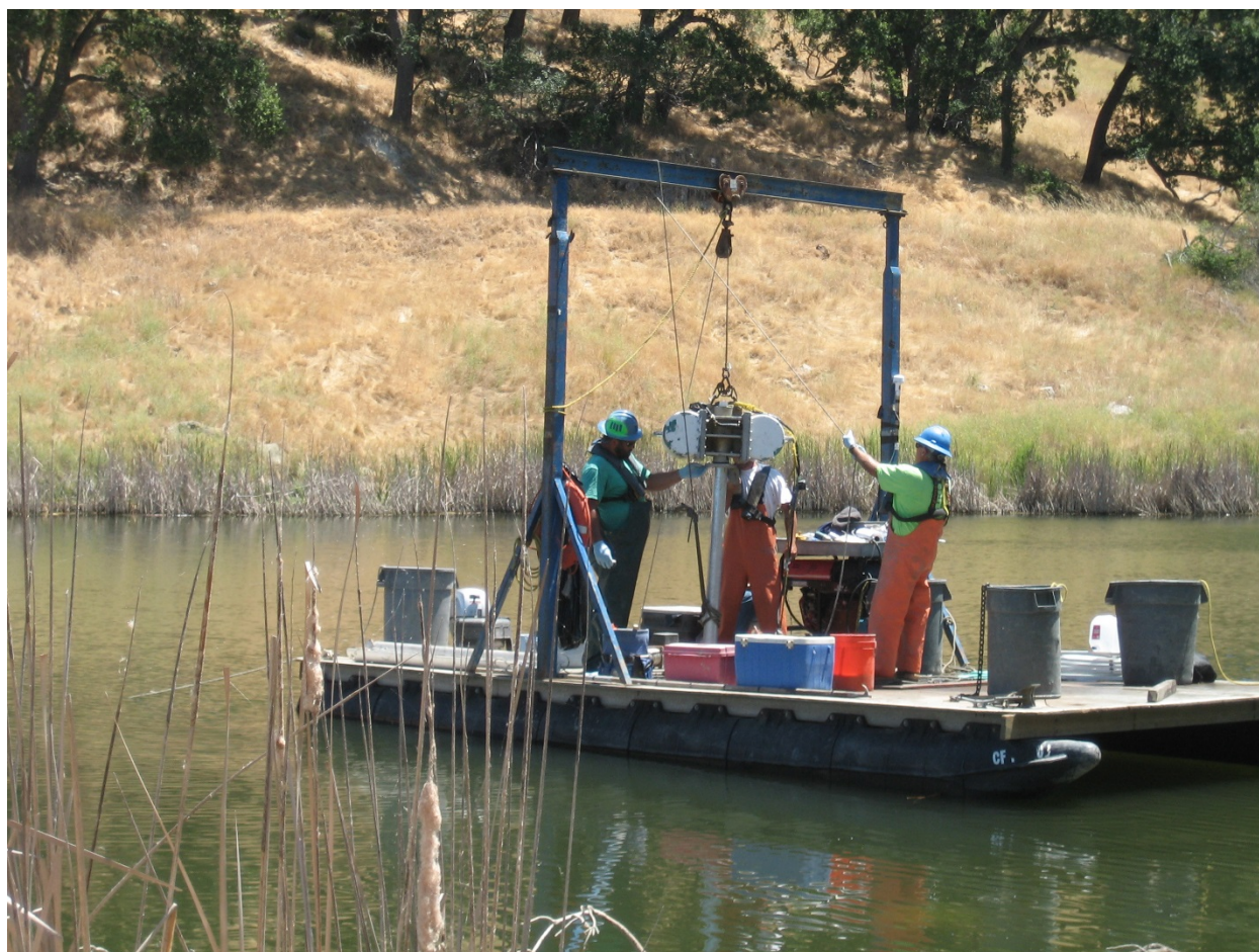
Figure 2. Vibroseise sampler at the Buena Vista Mercury Mine pond.
