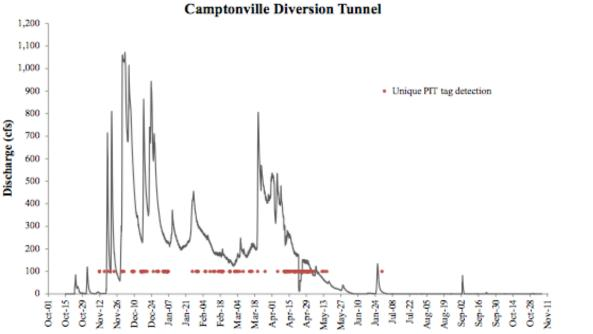
Figure 2.1.4-1. Flow and detections at Camptonville Diversion Tunnel. Note that maximum diversion capacity is 1,100 cfs.
