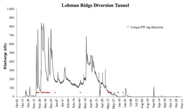
Figure 2.1.4-2. Flow and detections at Lohman Diversion Tunnel. Note that maximum diversion capacity is 860 cfs.
