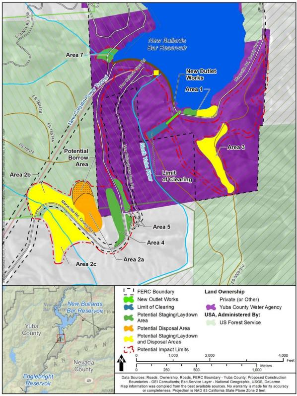
Figure 2.2.3-1. Conceptual layout of YCWA's proposed new Flood Control Outlet and areas that would be affected by construction of the outlet. [*from* Figure 2.2-5 in Exhibit E in YCWA's December 2, 2013 DLA.]
