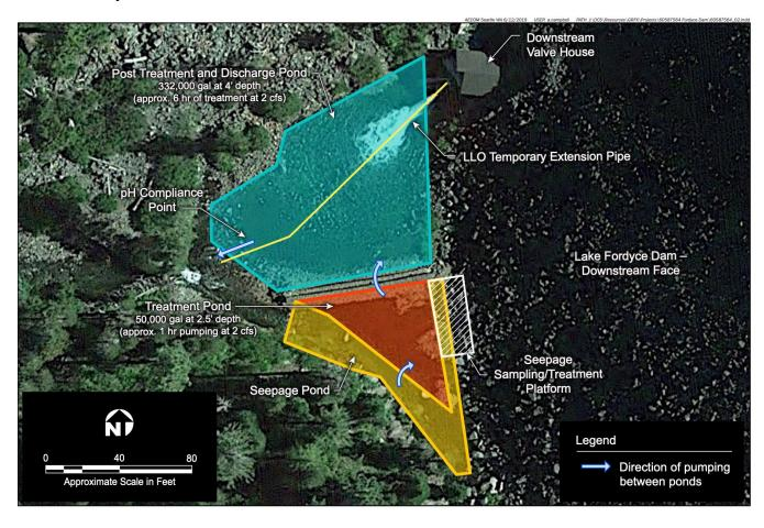
Figure 3. Downstream pH Control Configuration
