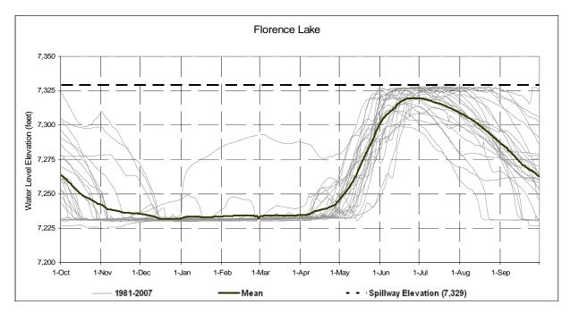
Figure 3-2. Florence Lake reservoir water levels 1981 to 2007. (Source: SCE, 2007a; USGS, 2008)
