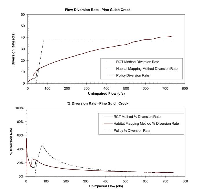
Figure A-7b. Diversion-impaired flow rating curves calculated for the Pine Gulch Creek validation site. The upper graph is the flow rate diverted in cfs, the lower graph is the corresponding percent of unimpaired flow diverted for the three diversion scenarios evaluated and graphed in Figure A-6a.
