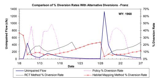
Figure A-24a. Example application of the method proposed by TU/WB/ESH for calculating diversion rate during a high flow event in the Franz Creek validation site. Diversion rates and resulting impaired flows are calculated for the Policy and the two alternative spawning flow methods proposed by TU/WB/ESH.
