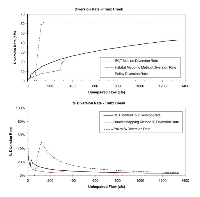
Figure A-12b. Diversion-impaired flow rating curves calculated for the Franz Creek validation site. The upper graph is the flow rate diverted in cfs, the lower graph is the corresponding percent of unimpaired flow diverted for the three diversion scenarios evaluated and graphed in Figure A-11a.
