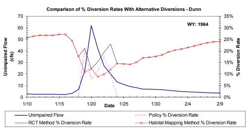
Figure A-15a. Example application of the method proposed by TU/WB/ESH for calculating diversion rate during a high flow event in the Dunn Creek validation site. Diversion rates and resulting impaired flows are calculated for the Policy and the two alternative spawning flow methods proposed by TU/WB/ESH.
