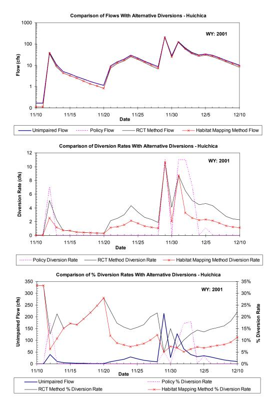
Figure A-17b. Another example application of the method proposed by TU/WB/ESH for calculating diversion rate during a high flow event in the Huichica Creek validation site. Diversion rates and resulting impaired flows are calculated for the Policy and the two alternative spawning flow methods proposed by TU/WB/ESH.
