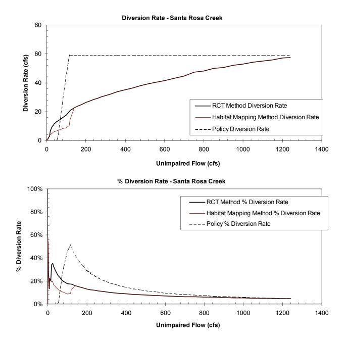
Figure A-9b. Diversion-impaired flow rating curves calculated for the Santa Rosa Creek validation site. The upper graph is the flow rate diverted in cfs, the lower graph is the corresponding percent of unimpaired flow diverted for the three diversion scenarios evaluated and graphed in Figure A-8a.
