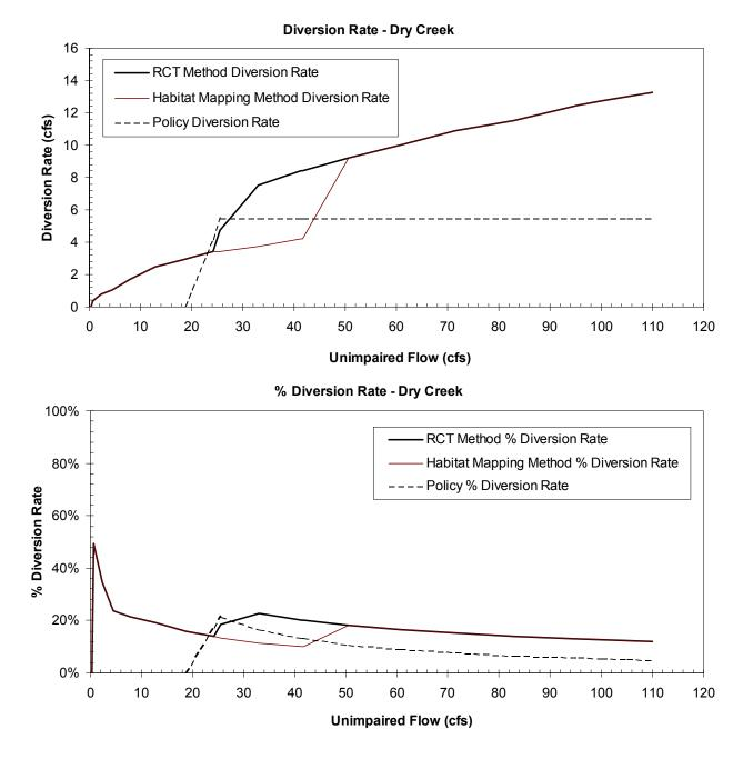
Figure A-2b. Diversion-impaired flow rating curves calculated for the Dry Creek validation site. The upper graph is the flow rate diverted in cfs, the lower graph is the corresponding percent of unimpaired flow diverted for the three diversion scenarios evaluated and graphed in Figure A-1a.
