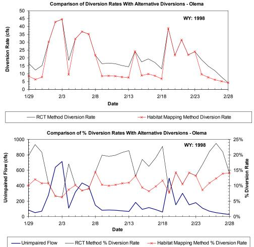
Figure A-18a. Example application of the method proposed by TU/WB/ESH for calculating diversion rate during a high flow event in the Olema Creek validation site. Diversion rates and resulting impaired flows are calculated for the two alternative spawning flow methods proposed by TU/WB/ESH.
