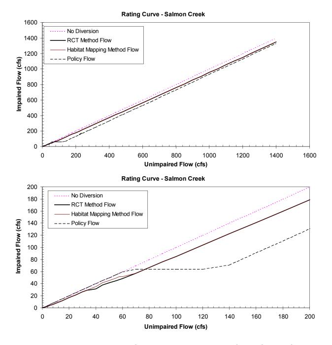
Figure A-11a. Impaired-unimpaired flow rating curves calculated for the Salmon Creek validation site. No diversion corresponds to the 1:1 line. The other lines are the resulting impaired flow resulting from implementation of (i) the draft Policy, and the TU/WB/ESH Proposal where the upper spawning flow threshold is determined using (ii) the RCT method, and (iii) the habitat mapping method. The lower graph is a blow-up of the upper graph in the low-flow image.
