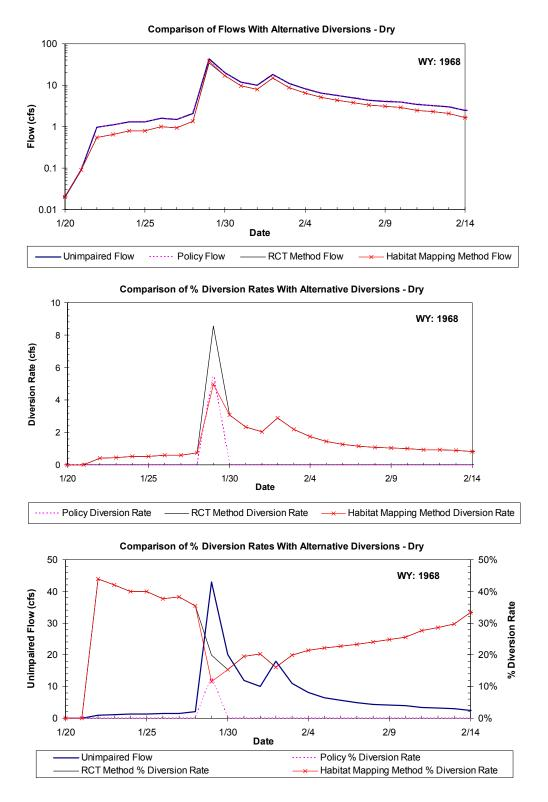
Figure A-14b. Another example application of the method proposed by TU/WB/ESH for calculating diversion rate during a high flow event in the Dry Creek validation site. Diversion rates and resulting impaired flows are calculated for the Policy and the two alternative spawning flow methods proposed by TU/WB/ESH.
