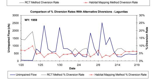
Figure A-25a. Example application of the method proposed by TU/WB/ESH for calculating diversion rate during a high flow event in the Lagunitas Creek validation site. Diversion rates and resulting impaired flows are calculated for the two alternative spawning flow methods proposed by TU/WB/ESH.
