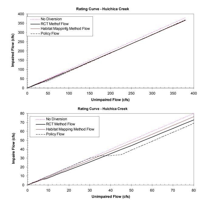
Figure A-5a. Impaired-unimpaired flow rating curves calculated for the Huichica Creek validation site. No diversion corresponds to the 1:1 line. The other lines are the resulting impaired flow resulting from implementation of (i) the draft Policy, and the TU/WB/ESH Proposal where the upper spawning flow threshold is determined using (ii) the RCT method, and (iii) the habitat mapping method. The lower graph is a blow-up of the upper graph in the low-flow image.
