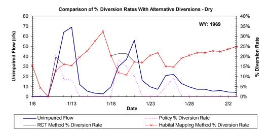
Figure A-14a. Example application of the method proposed by TU/WB/ESH for calculating diversion rate during a high flow event in the Dry Creek validation site. Diversion rates and resulting impaired flows are calculated for the Policy and the two alternative spawning flow methods proposed by TU/WB/ESH.
