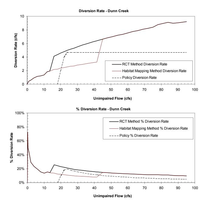
Figure A-3b. Diversion-impaired flow rating curves calculated for the Dunn Creek validation site. The upper graph is the flow rate diverted in cfs, the lower graph is the corresponding percent of unimpaired flow diverted for the three diversion scenarios evaluated and graphed in Figure A-2a.
