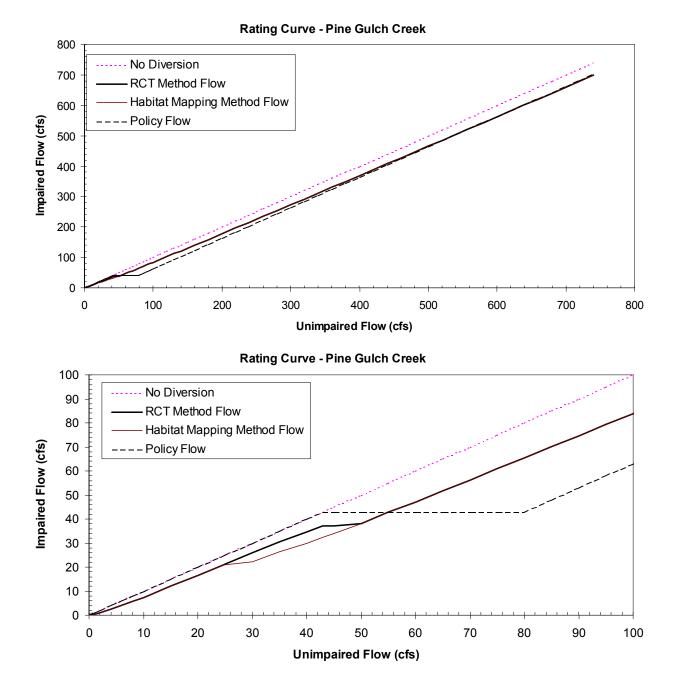
Figure A-7a. Impaired-unimpaired flow rating curves calculated for the Pine Gulch Creek validation site. No diversion corresponds to the 1:1 line. The other lines are the resulting impaired flow resulting from implementation of (i) the draft Policy, and the TU/WB/ESH Proposal where the upper spawning flow threshold is determined using (ii) the RCT method, and (iii) the habitat mapping method. The lower graph is a blow-up of the upper graph in the low-flow image.
