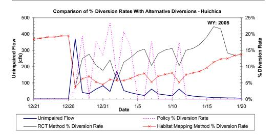
Figure A-17a. Example application of the method proposed by TU/WB/ESH for calculating diversion rate during a high flow event in the Huichica Creek validation site. Diversion rates and resulting impaired flows are calculated for the Policy and the two alternative spawning flow methods proposed by TU/WB/ESH.
