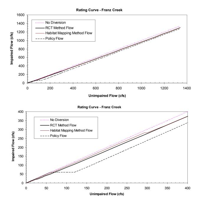
Figure A-12a. Impaired-unimpaired flow rating curves calculated for the Franz Creek validation site. No diversion corresponds to the 1:1 line. The other lines are the resulting impaired flow resulting from implementation of (i) the draft Policy, and the TU/WB/ESH Proposal where the upper spawning flow threshold is determined using (ii) the RCT method, and (iii) the habitat mapping method. The lower graph is a blow-up of the upper graph in the low-flow image.
