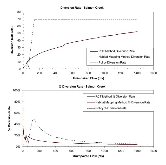
Figure A-11b. Diversion-impaired flow rating curves calculated for the Salmon Creek validation site. The upper graph is the flow rate diverted in cfs, the lower graph is the corresponding percent of unimpaired flow diverted for the three diversion scenarios evaluated and graphed in Figure A-10a.
