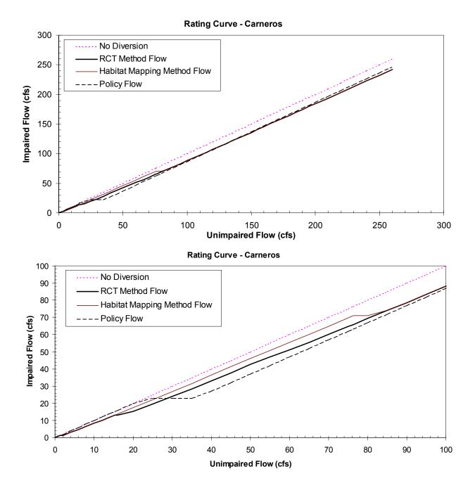
Figure A-4a. Impaired-unimpaired flow rating curves calculated for the Carneros Creek validation site. No diversion corresponds to the 1:1 line. The other lines are the resulting impaired flow resulting from implementation of (i) the draft Policy, and the TU/WB/ESH Proposal where the upper spawning flow threshold is determined using (ii) the RCT method, and (iii) the habitat mapping method. The lower graph is a blow-up of the upper graph in the low-flow image.
