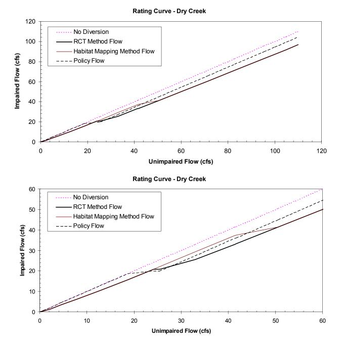
Figure A-2a. Impaired-unimpaired flow rating curves calculated for the Dry Creek validation site. No diversion corresponds to the 1:1 line. The other lines are the resulting impaired flow resulting from implementation of (i) the draft Policy, and the TU/WB/ESH Proposal where the upper spawning flow threshold is determined using (ii) the RCT method, and (iii) the habitat mapping method. The lower graph is a blow-up of the upper graph in the low-flow image.
