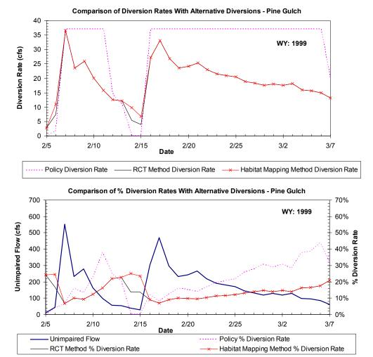
Figure A-19a. Example application of the method proposed by TU/WB/ESH for calculating diversion rate during a high flow event in the Pine Gulch Creek validation site. Diversion rates and resulting impaired flows are calculated for the Policy and the two alternative spawning flow methods proposed by TU/WB/ESH.
