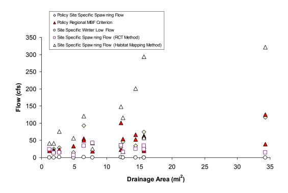
Figure A-1. Comparison of site-specific flows estimated for the validation sites following the procedures laid out in the TU/WB/ESH Proposal with the site specific steelhead spawning flows developed from site specific data and used in the development of the regional regression, and the corresponding regression estimates that would be applied if site specific data were unavailable.
