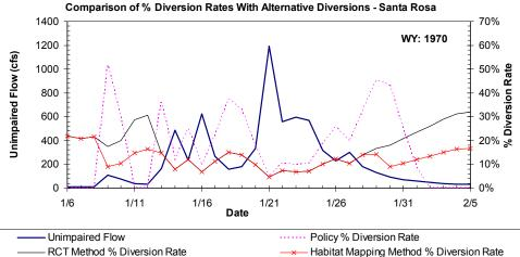
Figure A-21a. Example application of the method proposed by TU/WB/ESH for calculating diversion rate during a high flow event in the Santa Rosa Creek validation site. Diversion rates and resulting impaired flows are calculated for the Policy and the two alternative spawning flow methods proposed by TU/WB/ESH.
