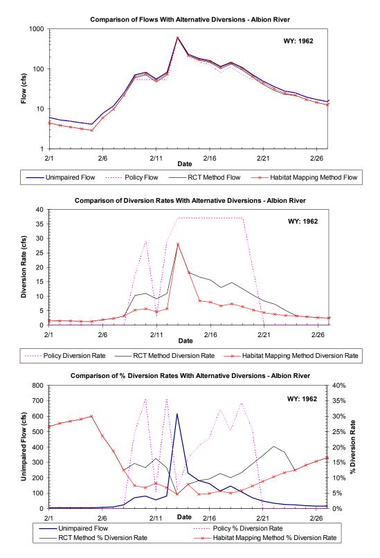
Figure A-22a. Example application of the method proposed by TU/WB/ESH for calculating diversion rate during a high flow event in the Albion River validation site. Diversion rates and resulting impaired flows are calculated for the Policy and the two alternative spawning flow methods proposed by TU/WB/ESH.
