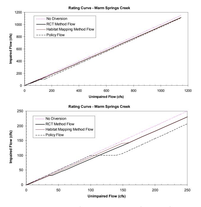
Figure A-8a. Impaired-unimpaired flow rating curves calculated for the Warm Springs Creek validation site. No diversion corresponds to the 1:1 line. The other lines are the resulting impaired flow resulting from implementation of (i) the draft Policy, and the TU/WB/ESH Proposal where the upper spawning flow threshold is determined using (ii) the RCT method, and (iii) the habitat mapping method. The lower graph is a blow-up of the upper graph in the low-flow image.
