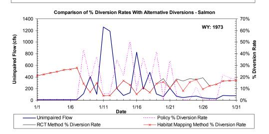
Figure A-23a. Example application of the method proposed by TU/WB/ESH for calculating diversion rate during a high flow event in the Salmon Creek validation site. Diversion rates and resulting impaired flows are calculated for the Policy and the two alternative spawning flow methods proposed by TU/WB/ESH.
