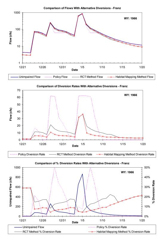
Figure A-24b. Another example application of the method proposed by TU/WB/ESH for calculating diversion rate during a high flow event in the Franz Creek validation site. Diversion rates and resulting impaired flows are calculated for the Policy and the two alternative spawning flow methods proposed by TU/WB/ESH.
