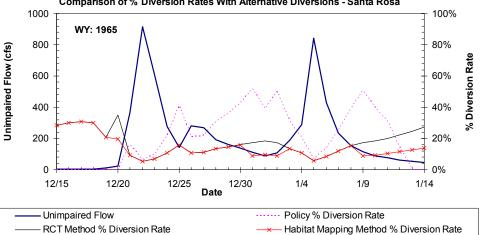
Figure A-21b. Another example application of the method proposed by TU/WB/ESH for calculating diversion rate during a high flow event in the Santa Rosa Creek validation site. Diversion rates and resulting impaired flows are calculated for the Policy and the two alternative spawning flow methods proposed by TU/WB/ESH.
