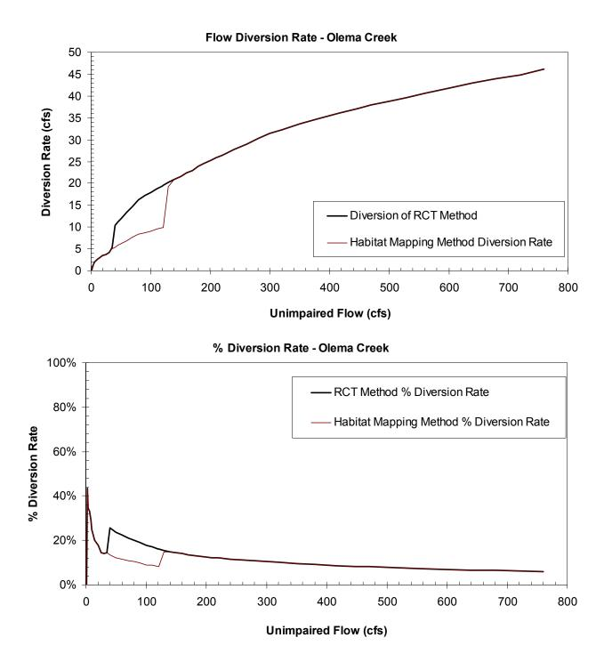
Figure A-6b. Diversion-impaired flow rating curves calculated for the Olema Creek validation site. The upper graph is the flow rate diverted in cfs, the lower graph is the corresponding percent of unimpaired flow diverted for the two diversion scenarios evaluated and graphed in Figure A-5a.
