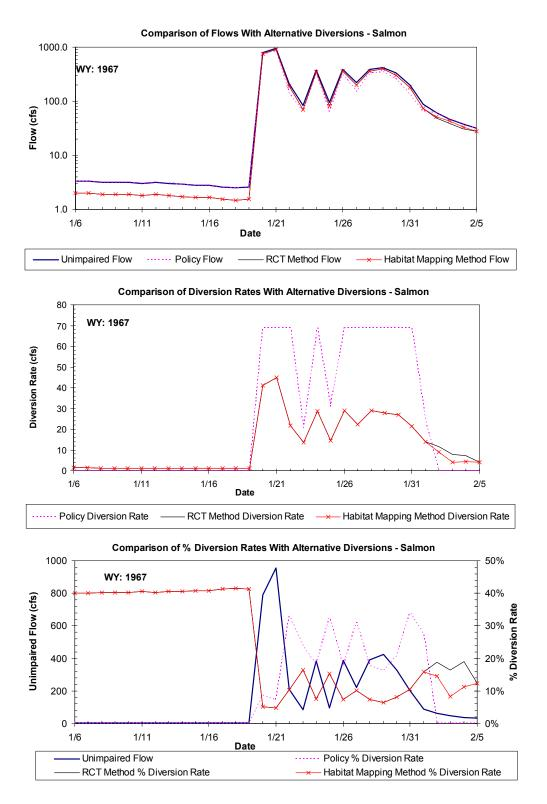
Figure A-23b. Another example application of the method proposed by TU/WB/ESH for calculating diversion rate during a high flow event in the Salmon Creek validation site. Diversion rates and resulting impaired flows are calculated for the Policy and the two alternative spawning flow methods proposed by TU/WB/ESH.
