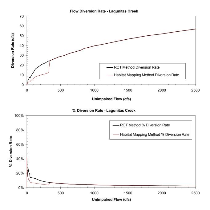
Figure A-13b. Diversion-impaired flow rating curves calculated for the Lagunitas Creek validation site. The upper graph is the flow rate diverted in cfs, the lower graph is the corresponding percent of unimpaired flow diverted for the two diversion scenarios evaluated and graphed in Figure A-12a.
