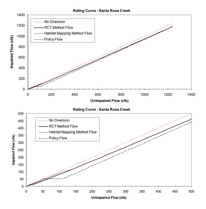
Figure A-9a. Impaired-unimpaired flow rating curves calculated for the Santa Rosa Creek validation site. No diversion corresponds to the 1:1 line. The other lines are the resulting impaired flow resulting from implementation of (i) the draft Policy, and the TU/WB/ESH Proposal where the upper spawning flow threshold is determined using (ii) the RCT method, and (iii) the habitat mapping method. The lower graph is a blow-up of the upper graph in the low-flow image.
