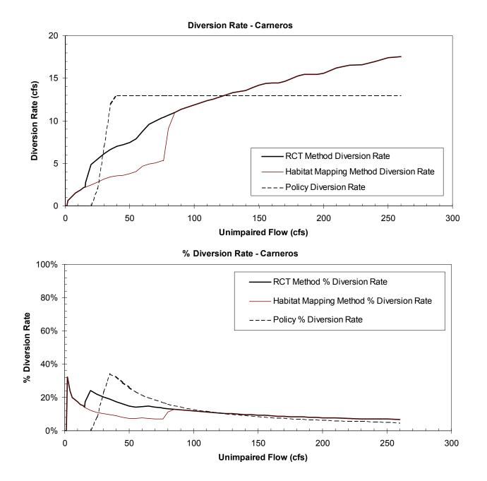
Figure A-4b. Diversion-impaired flow rating curves calculated for the Carneros Creek validation site. The upper graph is the flow rate diverted in cfs, the lower graph is the corresponding percent of unimpaired flow diverted for the three diversion scenarios evaluated and graphed in Figure A-3a.
