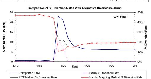
Figure A-15b. Another example application of the method proposed by TU/WB/ESH for calculating diversion rate during a high flow event in the Dunn Creek validation site. Diversion rates and resulting impaired flows are calculated for the Policy and the two alternative spawning flow methods proposed by TU/WB/ESH.
