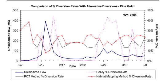
Figure A-19b. Another example application of the method proposed by TU/WB/ESH for calculating diversion rate during a high flow event in the Pine Gulch Creek validation site. Diversion rates and resulting impaired flows are calculated for the Policy and the two alternative spawning flow methods proposed by TU/WB/ESH.
