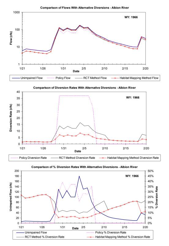
Figure A-22b. Another example application of the method proposed by TU/WB/ESH for calculating diversion rate during a high flow event in the Albion River validation site. Diversion rates and resulting impaired flows are calculated for the Policy and the two alternative spawning flow methods proposed by TU/WB/ESH.
