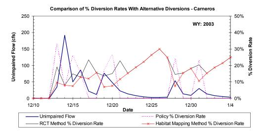
Figure A-16b. Another example application of the method proposed by TU/WB/ESH for calculating diversion rate during a high flow event in the Carneros Creek validation site. Diversion rates and resulting impaired flows are calculated for the Policy and the two alternative spawning flow methods proposed by TU/WB/ESH.
