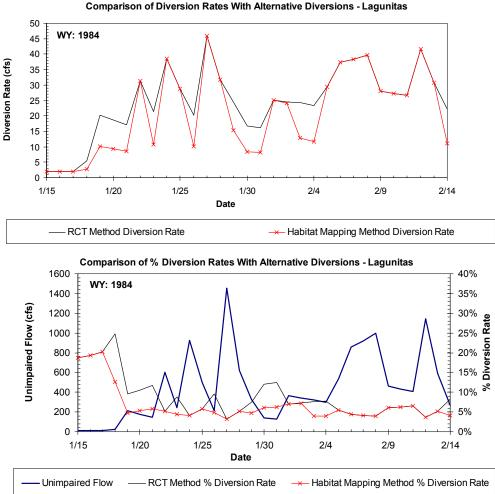
Figure A-25b. Another example application of the method proposed by TU/WB/ESH for calculating diversion rate during a high flow event in the Lagunitas Creek validation site. Diversion rates and resulting impaired flows are calculated for the two alternative spawning flow methods proposed by TU/WB/ESH.
