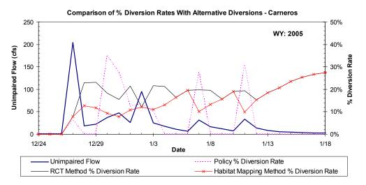
Figure A-16a. Example application of the method proposed by TU/WB/ESH for calculating diversion rate during a high flow event in the Carneros Creek validation site. Diversion rates and resulting impaired flows are calculated for the Policy and the two alternative spawning flow methods proposed by TU/WB/ESH.
