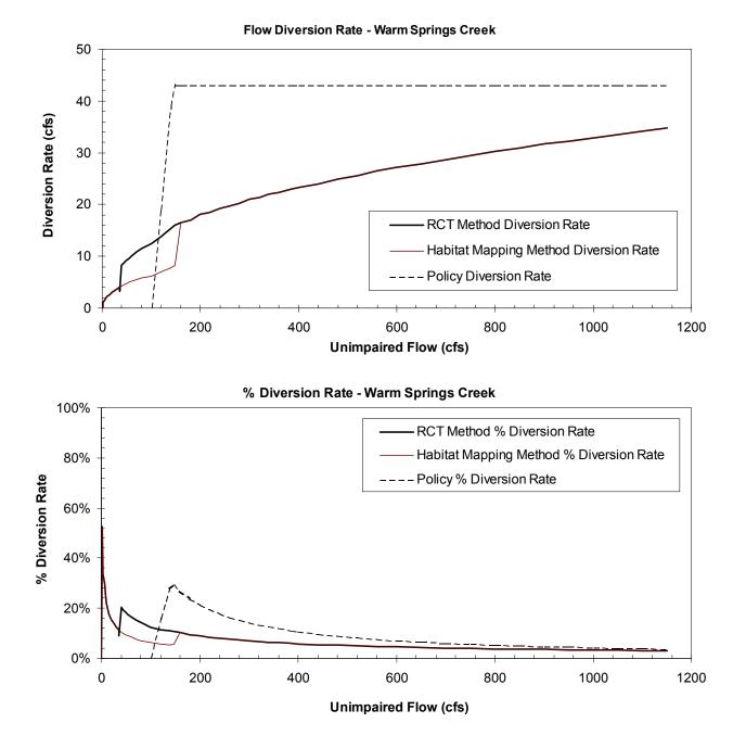
Figure A-8b. Diversion-impaired flow rating curves calculated for the Warm Springs Creek validation site. The upper graph is the flow rate diverted in cfs, the lower graph is the corresponding percent of unimpaired flow diverted for the three diversion scenarios evaluated and graphed in Figure A-7a.
