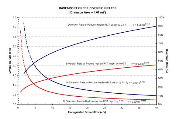
*Figure 10. Fixed diversion rates as a function of unregulated streamflows for Davenport Creek at 0.10 ft and 0.05 ft diversion rates.*
