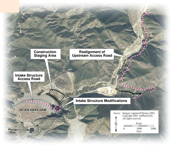
Project-related construction activities at Seven Oaks Dam would be spread over three summers. Construction would be planned so that it would be completed within the non-flood season and, thus, would not impair the flood control function of the facility.
