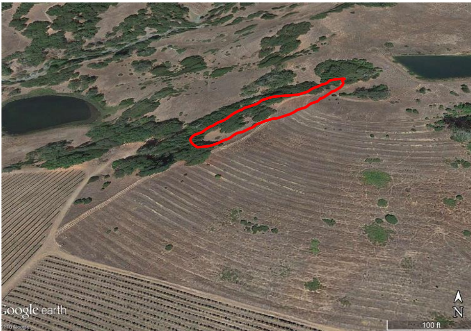
Figure 9. The red polygon depicts where fill was placed into the unnamed tributary to Maple Creek. Placement of fill materials has substantially changed the bank of the stream, see FGC section 1602 and 5650. In addition, tile drains have been installed within the terraced hillside (every 5 terraces, Mr. Peters, Personal Communication) and directly concentrated run-off to the stream channel, see FGC section 1602.
