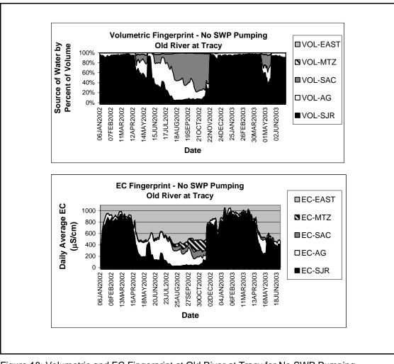
Figure 18: Volumetric and EC Fingerprint at Old River at Tracy for No SWP Pumping Simulation, Jan 2002 – July 2003
