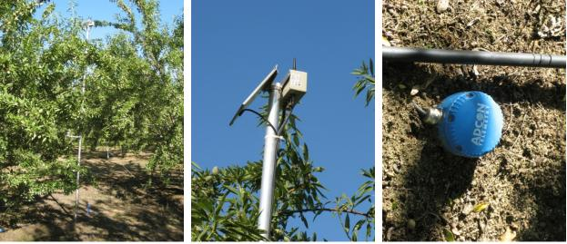
ADCON Soil Moisture and Weather Monitoring Station.
