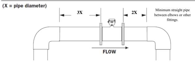
Figure 1. Example Magnetic Flow Meter Installation.
