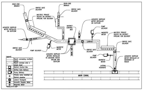
Figure A-7. Typical laterals conveying multiple and single heads with pump, multiple valve, and orifice gate turnouts and flow measurement network delivery measurement devices.
