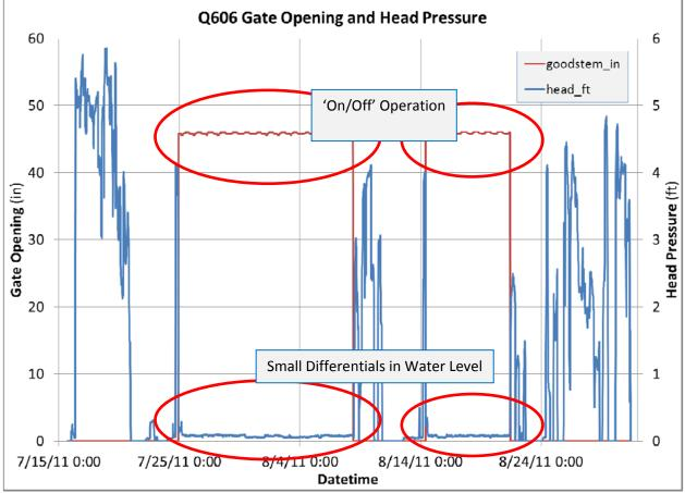
Figure A-6. Orifice gate water level differential measurements.
