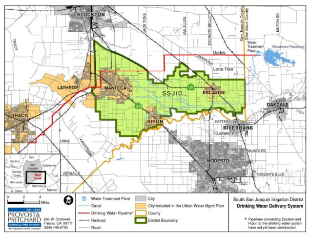
Figure 5-5. SCWSP Phase I Water System
