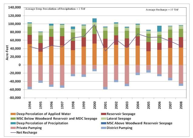
Figure 5-6. Groundwater System Inflows, Outflows, and Net Recharge, 1994 to 2008
