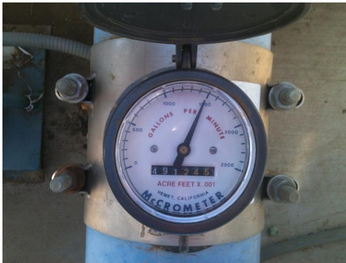
saddle propeller meter Figure F-8 Testing of a Water Specialties saddle propeller meter using PT878 with a stand pipe configuration.
