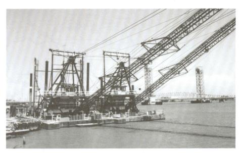
Typical bargemounted crane used for levee maintenance.
