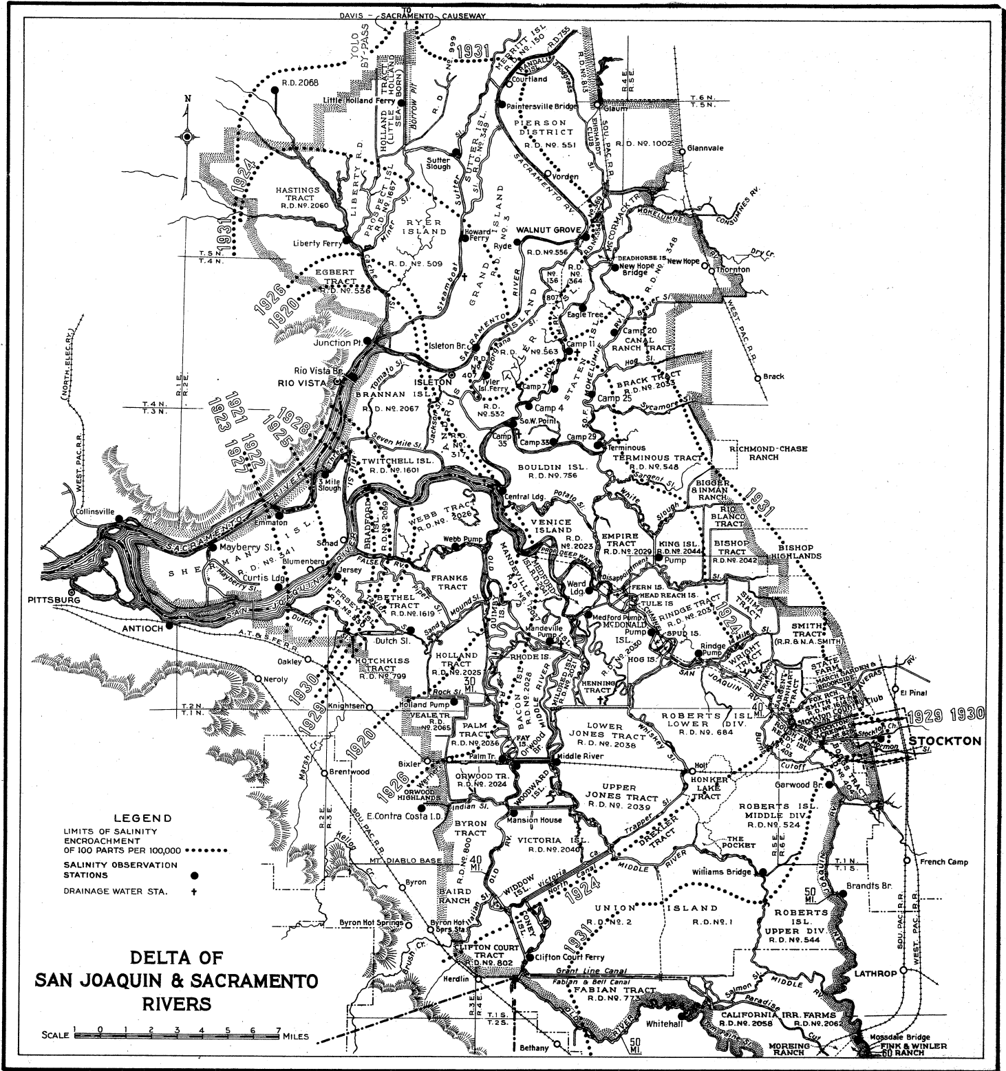
MAXIMUM SEASONAL SALINITY ENCROACHMENT OF 100 PARTS OF CHLORINE PER 100,000 PARTS OF WATER, SACRAMENTO-SAN JOAQUIN DELTA, 1920-1931
