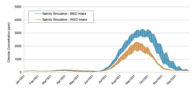
Figure 6-5. Simulated chloride concentrations at the BBID and WSID intakes
