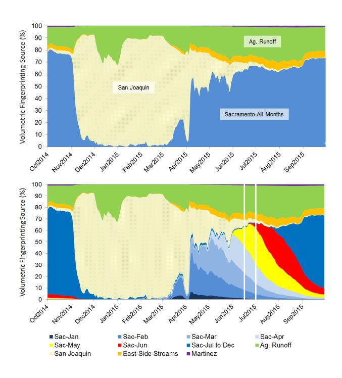
Figure 6-12 Source fingerprints for water at WSID intake for water year 2015 (a), and showing the month when Sacramento River water entered the Delta (b)
