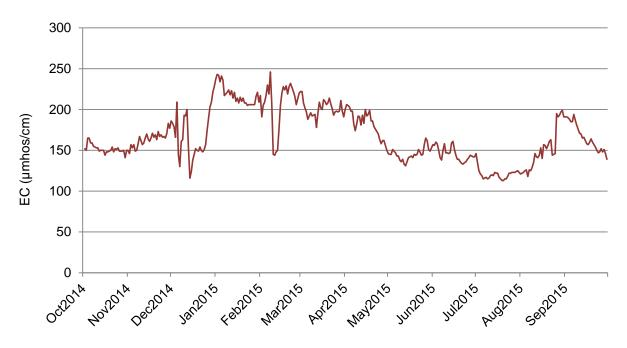
Figure A-14 EC of Sacramento River at Freeport and Yolo Bypass (Source: CDEC)
