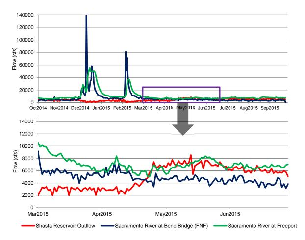
Figure 5-10. Shasta Reservoir outflow, Sacramento River FNF at Bend Bridge, and Sacramento River at Freeport during the 2014/2015 water year (top), and the same comparison focused on the point where reservoir outflow surpasses FNF at Bend Bridge (bottom). Note the change in scales on x and y-axes between top and bottom graphs (FNF Data and Shasta Reservoir Outflow from CDEC, accessed online 1-5-2015)
