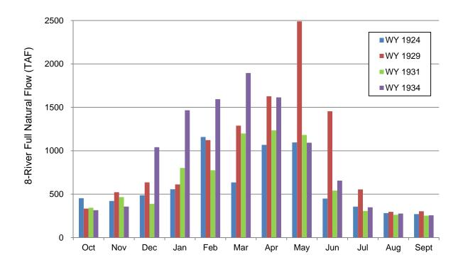
Figure 5-1. 8-River index FNF during pre-CVP/SWP critical water years (Data from DWR Bulletin 23 documents; DWR 1930a, DWR 1930b, DWR 1932, DWR 1935)
