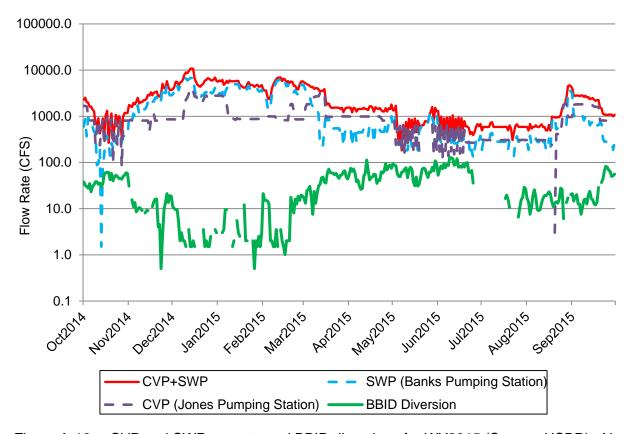
Figure A-16. CVP and SWP exports, and BBID diversions for WY2015 (Source: USBR). Note the log-scale.
