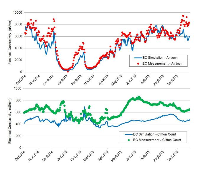
Figure 6-9. Modeled and measured EC at Antioch (a) and at Clifton Court Forebay (b) during WY 2015 (measured data from CDEC, accessed 11-20-2015)
