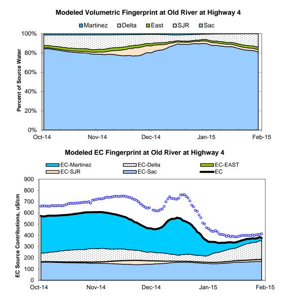
Figure 4-10. Source fingerprinting by volume (top) and EC (bottom) in Old River at Highway 4 between October 2014 and February 2015 (Data collected and plotted by DWR; obtained online at www.water.ca.gov on 1-6-2016)
