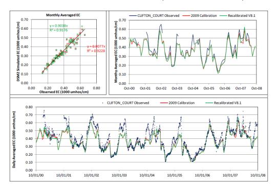
Figure 6-3. DSM2 EC calibration results at Clifton Court (DWR 2013a and 2013b)
