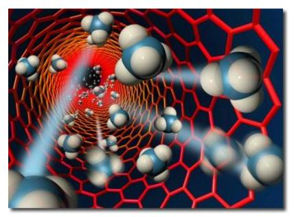
The nanotubes, special molecules made of carbon atoms in a unique arrangement, are hollow and more than 50.000 times thinner than a human hair. Billions of these tubes act as the pores in the membrane. The super smooth inside of the nanotubes allow liquids and gases to rapidly flow through, while the tiny pore size can block larger molecules. This previously unobserved phenomenon opens a vast array of possible applications.
