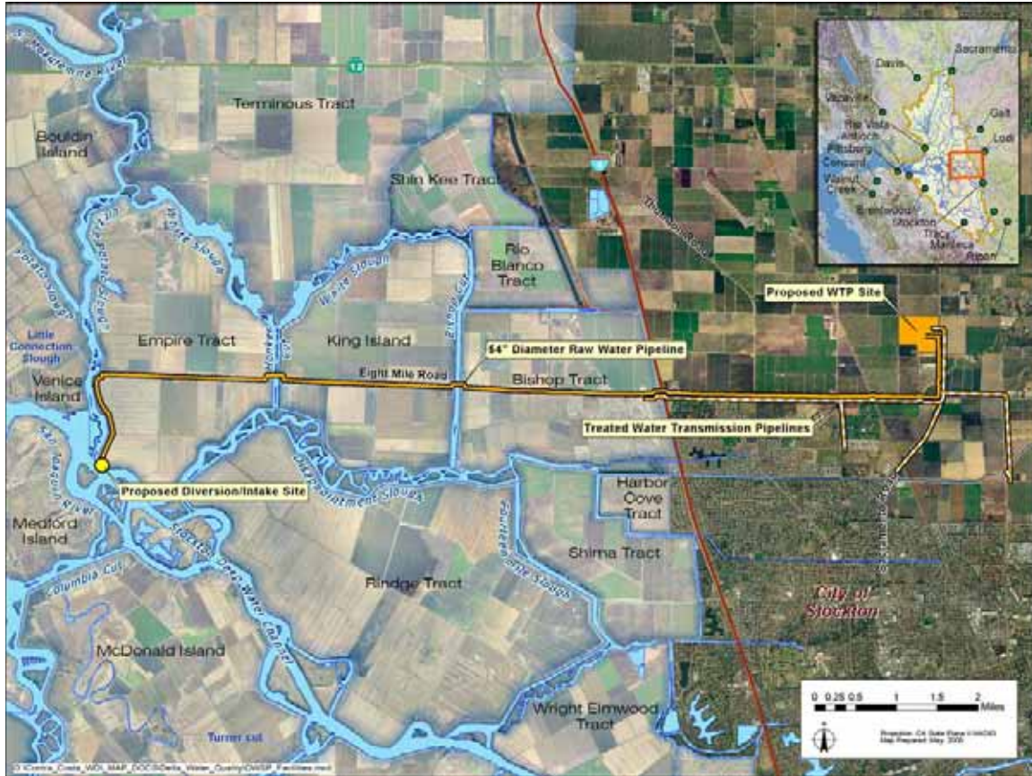
Figure 4-13 Facilities for the Delta Water Supply Project
