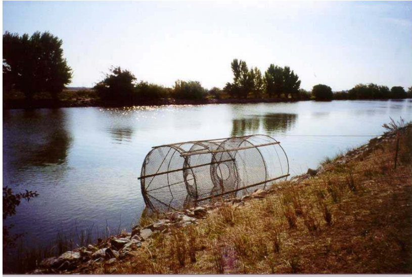
Figure 5. Picture of a fyke trap used to collect adult Chinook salmon (and other fish) in the Delta Cross Channel, Georgiana Slough, and Sacramento River, California (4 September through 15 November 2001).
