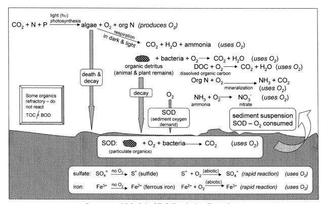
Conceptual Model of DO Depletion Reactions in the SJR DWSC
