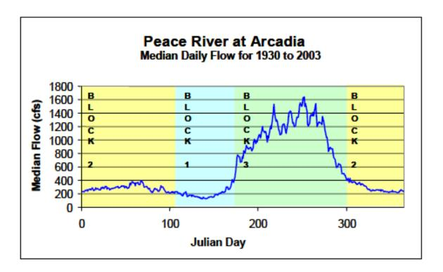
Figure 4. Median daily flow at Peace River at Arcadia, FL. with hydrograph separated into high, median and low flow blocks.
