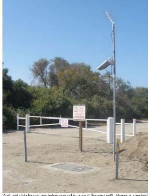
Well and data logger are below-ground in a vault (foreground). Power is supplied by a solar panel on the pole, and data are transmitted via satellite using the antenna on top of the pole.
