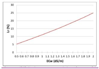
**Figure 1.** Alfalfa leaching requirement (Lr) as a function of the average applied water (ECa).<u>salinity</u> (ECw).
