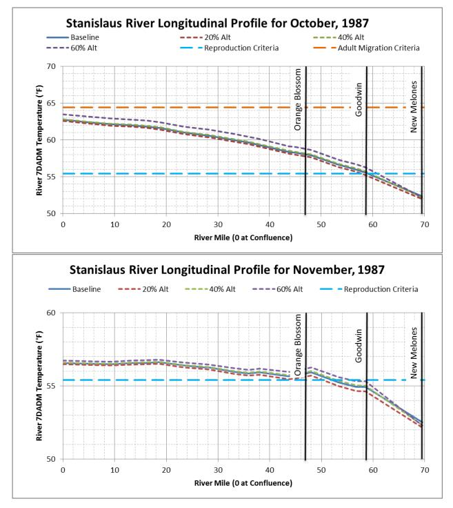
Figure F.1.6-14. Longitudinal Monthly Average 7DADM Temperature Results within the Stanislaus River for (a) October 1987 and (b) November 1987
