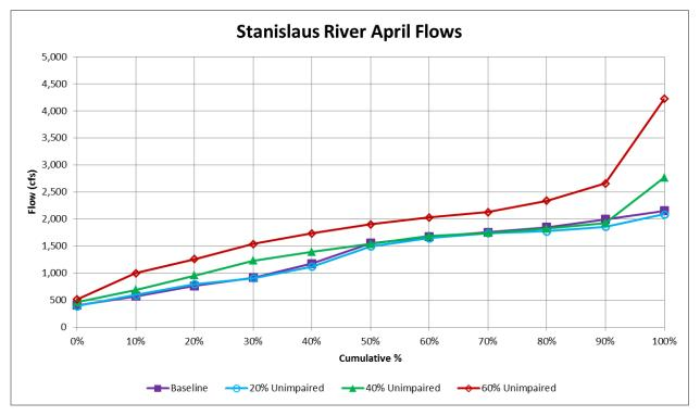
Figure F.1.4-3d. WSE-Simulated Cumulative Distributions of Stanislaus River April Flows (cfs) at Ripon for Baseline Conditions and 20%, 40%, 60% Unimpaired Flow (LSJR Alternatives 2–4)
