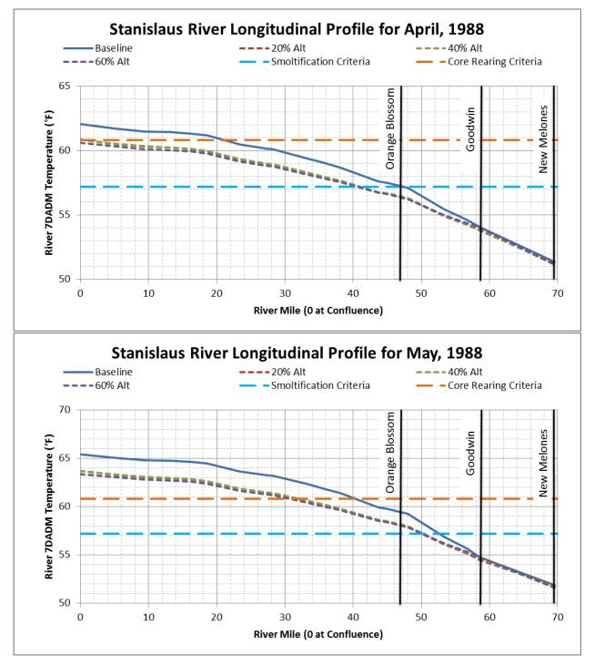
Figure F.1.6-17. Longitudinal Monthly Average 7DADM Temperature Results within the Stanislaus River for (a) April 1988 and (b) May 1988
