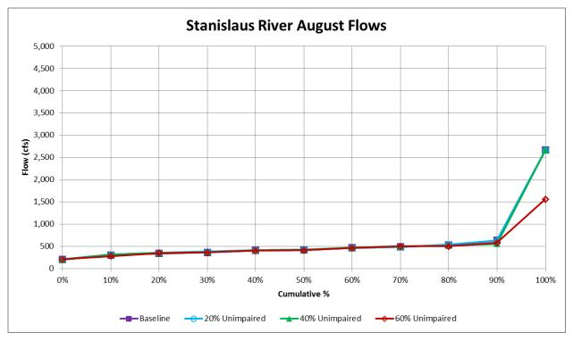
Figure F.1.4-3h. WSE-Simulated Cumulative Distributions of Stanislaus River August Flows (cfs) at Ripon for Baseline Conditions and 20%, 40%, 60% Unimpaired Flow (LSJR Alternatives 2–4)
