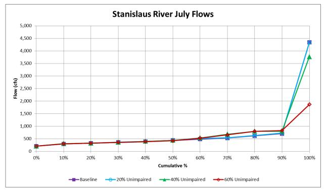
Figure F.1.4-3g. WSE-Simulated Cumulative Distributions of Stanislaus River July Flows (cfs) at Ripon for Baseline Conditions and 20%, 40%, 60% Unimpaired Flow (LSJR Alternatives 2-4)
