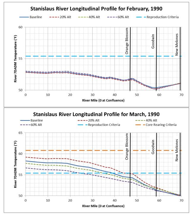
Figure F.1.6-22. Longitudinal Monthly Average 7DADM Temperature Results within the Stanislaus River for (a) February 1990 and (b) March 1990
