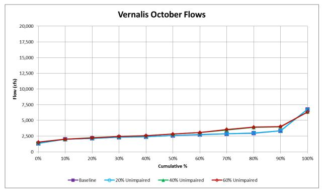
Figure F.1.4-4j. WSE-Simulated Cumulative Distributions of SJR at Vernalis October Flows (cfs) for Baseline Conditions and 20%, 40%, 60% Unimpaired Flow (LSJR Alternatives 2-4)
