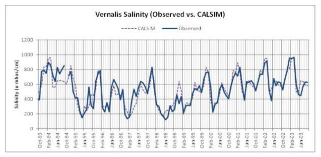
Figure F.1.5-1. Comparison of CALSIM II Salinity Output at Vernalis to Monthly Average Observed Data at the Same Location for Water Years 1994–2003)
