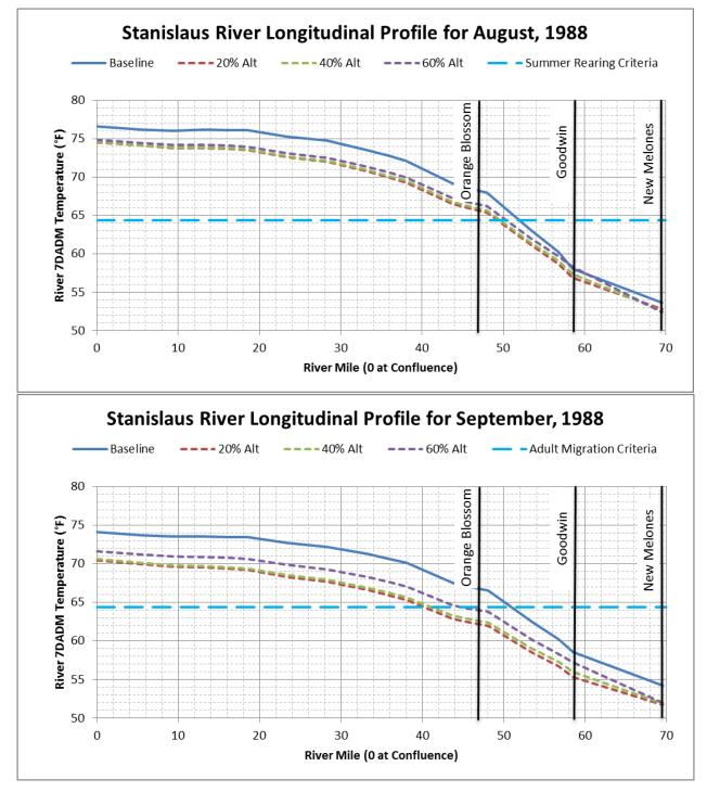
Figure F.1.6-19. Longitudinal Monthly Average 7DADM Temperature Results within the Stanislaus River for (a) August 1988 and (b) September 1988
