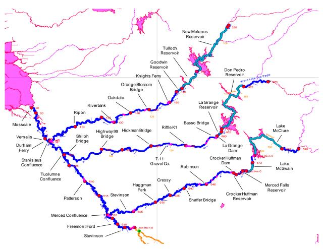
Figure F.1.6-1. The SJR Basin, Including the Stanislaus, Tuolumne, and Merced River Systems, as Represented in the HEC-5Q Model
