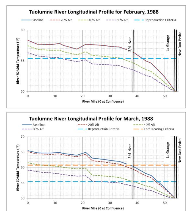
Figure F.1.6-34. Longitudinal Monthly Average 7DADM Temperature Results within the Tuolumne River for (a) February 1988 and (b) March 1988
