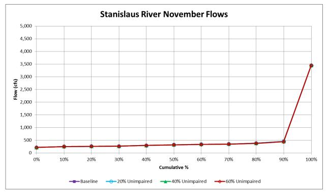
Figure F.1.4-3k. WSE-Simulated Cumulative Distributions of Stanislaus River November Flows (cfs) at Ripon for Baseline Conditions and 20%, 40%, 60% Unimpaired Flow (LSJR Alternatives 2–4)
