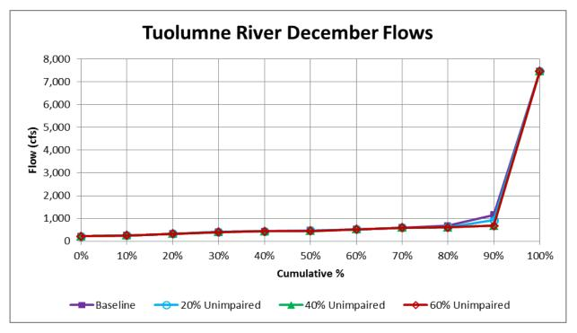
Figure F.1.4-2I. WSE-Simulated Cumulative Distributions of Tuolumne River December Flows (cfs) at Modesto for Baseline Conditions and 20%, 40%, 60% Unimpaired Flow (LSJR Alternatives 2-4)
