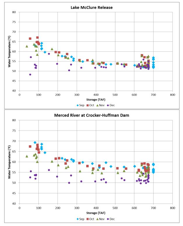
Figure F.1.6-7a. Effects of Lake McClure Storage on Lake McClure and Crocker-Huffman Release Temperatures September–December for Baseline Conditions 1970–2003
