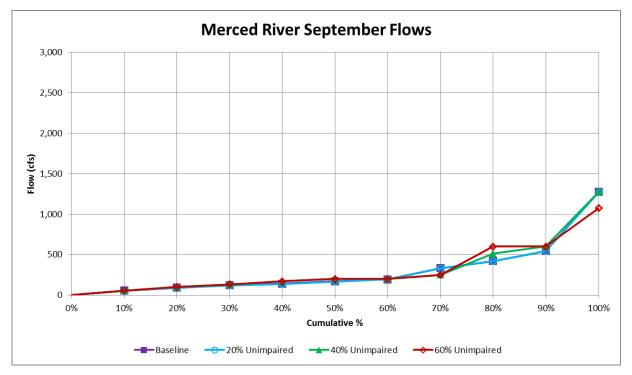
Figure F.1.4-1i. WSE-Simulated Cumulative Distributions of Merced River September Flows (cfs) at Stevinson for Baseline Conditions and 20%, 40%, 60% Unimpaired Flow (LSJR Alternatives 2–4)
