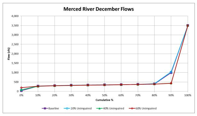
Figure F.1.4-1I. WSE-Simulated Cumulative Distributions of Merced River December Flows (cfs) at Stevinson for Baseline Conditions and 20%, 40%, 60% Unimpaired Flow (LSJR Alternatives 2–4)
