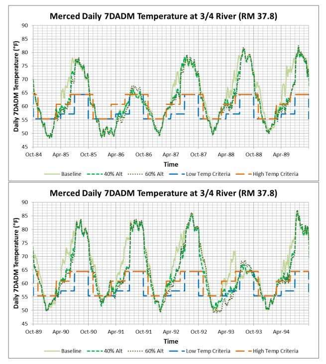
Figure F.1.6-49. Temperature Model 7DADM Results at Merced RM 37.8 Compared to Monthly USEPA Temperature Criteria for Optimal Development of Different Fish Lifestages under Baseline and LSJR Alternatives 2 and 3 (40% and 60% of Unimpaired Flow Feb-June) for (a) Water Years 1985-1989 and (b) Water Years 1990–1994
