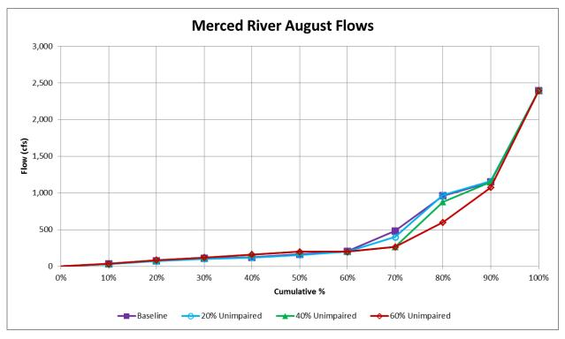
Figure F.1.4-1h. WSE-Simulated Cumulative Distributions of Merced River August Flows (cfs) at Stevinson for Baseline Conditions and 20%, 40%, 60% Unimpaired Flow (LSJR Alternatives 2–4)
