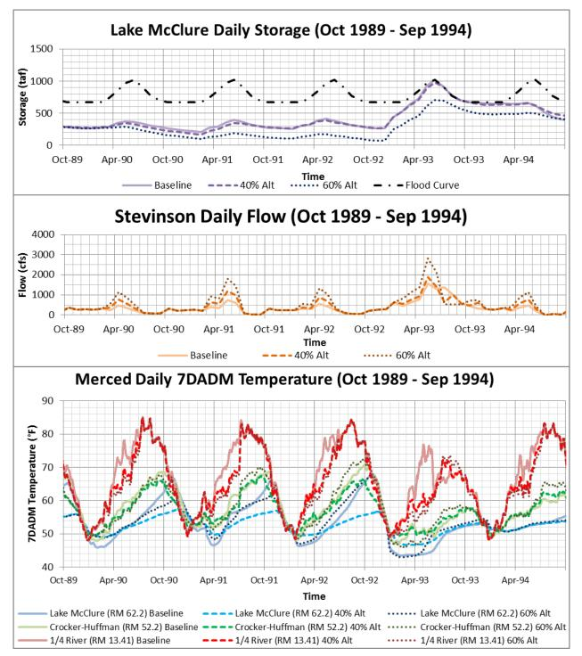
Figure F.1.6-46. Merced River Temperature Model Results for LSJR Alternatives 2 and 3 (40% and 60% of Unimpaired Flow Feb–June) and Baseline Scenarios for the Water Years 1990–1994, Showing (a) Reservoir Storage, (b) Instream Flows, and (c) Daily 7DADM Temperature at Lake McClure Release, Crocker-Huffman Dam Release, and 1/4 River Locations
