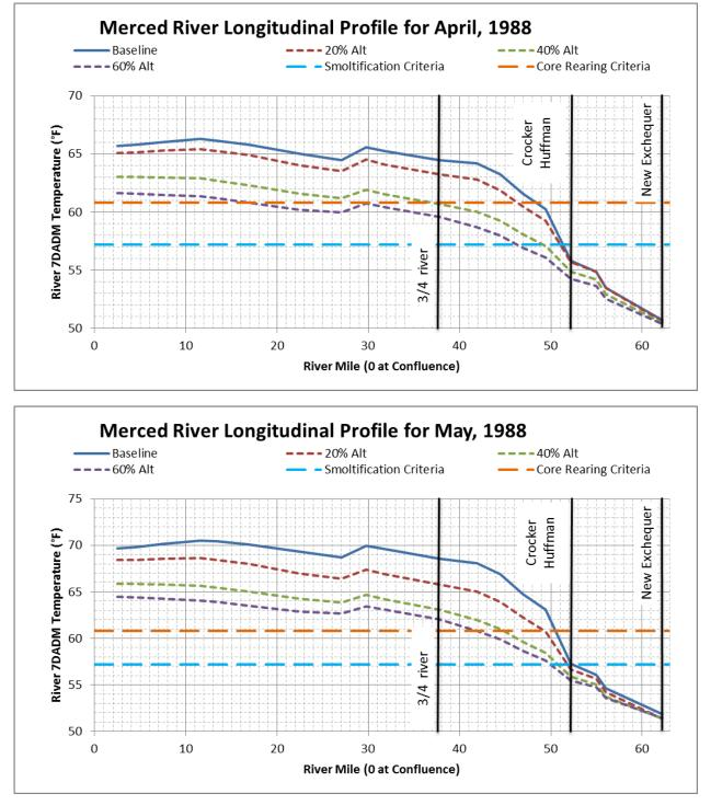
Figure F.1.6-53. Longitudinal Monthly Average 7DADM Temperature Results within the Merced River for (a) April 1988 and (b) May 1988
