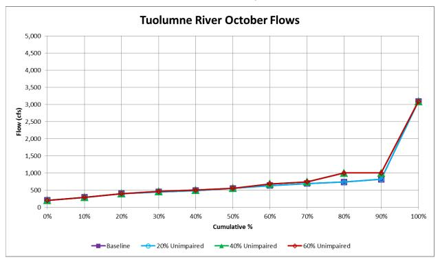
Figure F.1.4-2j. WSE-Simulated Cumulative Distributions of Tuolumne River October Flows (cfs) at Modesto for Baseline Conditions and 20%, 40%, 60% Unimpaired Flow (LSJR Alternatives 2–4)
