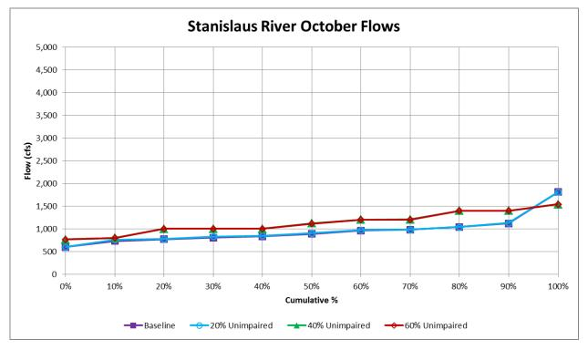
Figure F.1.4-3j. WSE-Simulated Cumulative Distributions of Stanislaus River October Flows (cfs) at Ripon for Baseline Conditions and 20%, 40%, 60% Unimpaired Flow (LSJR Alternatives 2–4)
