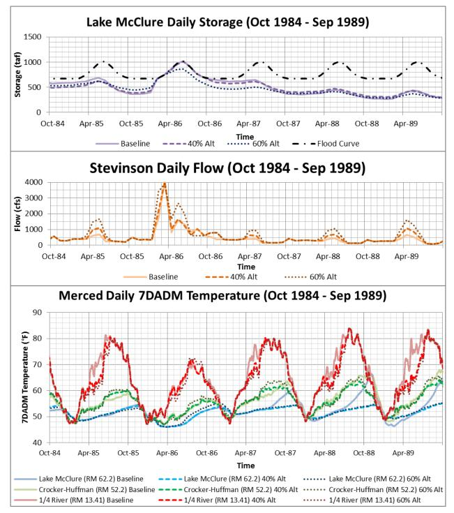
Figure F.1.6-45. Merced River Temperature Model Results for LSJR Alternatives 2 and 3 (40% and 60% of Unimpaired Flow Feb–June) and Baseline Scenarios for the Water Years 1985–1989, Showing (a) Reservoir Storage, (b) Instream Flows, and (c) Daily 7DADM Temperature at Lake McClure Release, Crocker-Huffman Dam Release, and 1/4 River Locations
