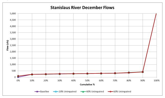
Figure F.1.4-3I. WSE-Simulated Cumulative Distributions of Stanislaus River December Flows (cfs) at Ripon for Baseline Conditions and 20%, 40%, 60% Unimpaired Flow (LSJR Alternatives 2-4)
