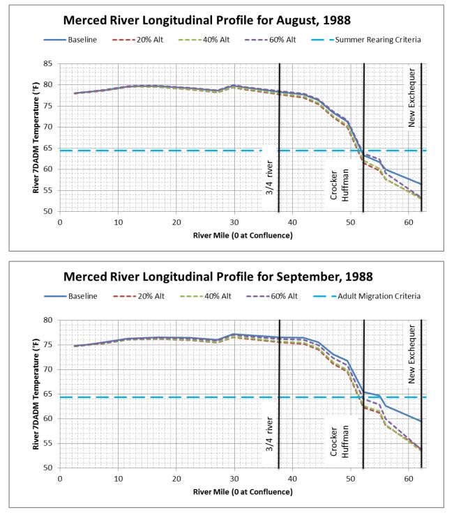
Figure F.1.6-55. Longitudinal Monthly Average 7DADM Temperature Results within the Merced River for (a) August 1988 and (b) September 1988
