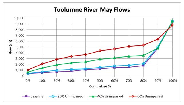
Figure F.1.4-2e. WSE-Simulated Cumulative Distributions of Tuolumne River May Flows (cfs) at Modesto for Baseline Conditions and 20%, 40%, 60% Unimpaired Flow (LSJR Alternatives 2–4)
