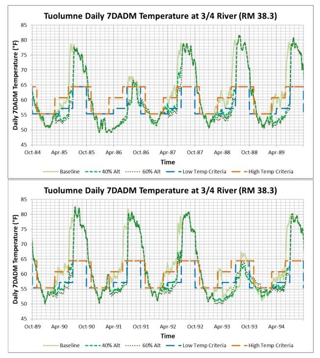
Figure F.1.6-31. Temperature Model 7DADM Results at Tuolumne RM 38.3 Compared to Monthly USEPA Temperature Criteria for Optimal Development of Different Fish Lifestages under Baseline and LSJR Alternatives 2 and 3 (40% and 60% of Unimpaired Flow Feb–June) for (a) Water Years 1985–1989 and (b) Water Years 1990-1994
