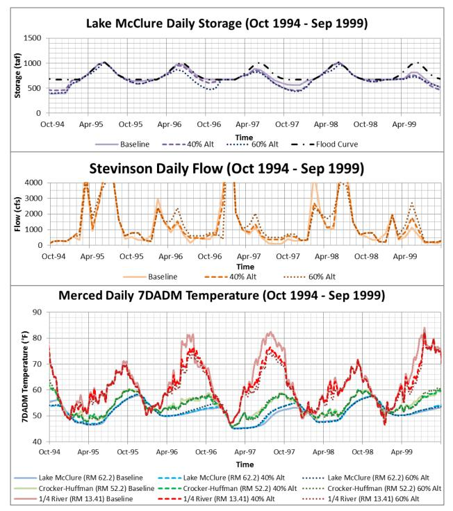
Figure F.1.6-47. Merced River Temperature Model Results for LSJR Alternatives 2 and 3 (40% and 60% of Unimpaired Flow Feb–June) and Baseline Scenarios for the Water Years 1995–1999, Showing (a) Reservoir Storage, (b) Instream Flows, and (c) Daily 7DADM Temperature at Lake McClure Release, Crocker-Huffman Dam Release, and 1/4 River Locations
