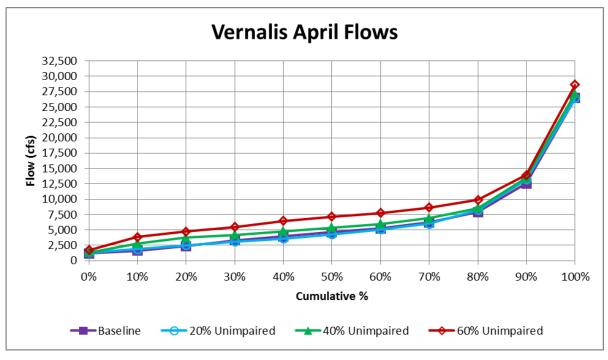
Figure F.1.4-4d. WSE-Simulated Cumulative Distributions of SJR at Vernalis April Flows (cfs) for Baseline Conditions and 20%, 40%, 60% Unimpaired Flow (LSJR Alternatives 2–4)
