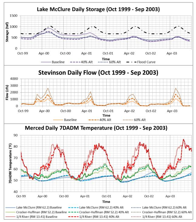
Figure F.1.6-48. Merced River Temperature Model Results for LSJR Alternatives 2 and 3 (40% and 60% of Unimpaired Flow Feb–June) and Baseline Scenarios for the Water Years 2000–2003, Showing (a) Reservoir Storage, (b) Instream Flows, and (c) Daily 7DADM Temperature at Lake McClure Release, Crocker-Huffman Dam Release, and 1/4 River Locations
