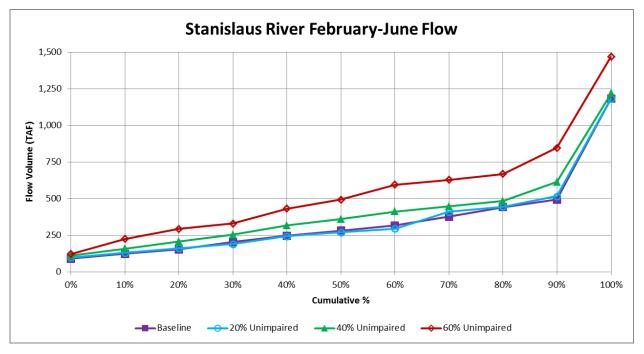
Figure F.1.4-3a. WSE-Simulated Cumulative Distributions of Stanislaus River February–June Flow Volumes (TAF) at Ripon for Baseline Conditions and 20%, 40%, 60% Unimpaired Flow (LSJR Alternatives 2-4)
