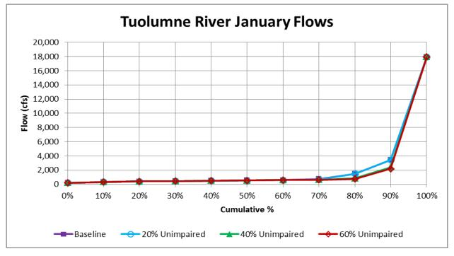
Figure F.1.4-2m. WSE-Simulated Cumulative Distributions of Tuolumne River January Flows (cfs) at Modesto for Baseline Conditions and 20%, 40%, 60% Unimpaired Flow (LSJR Alternatives 2–4)
