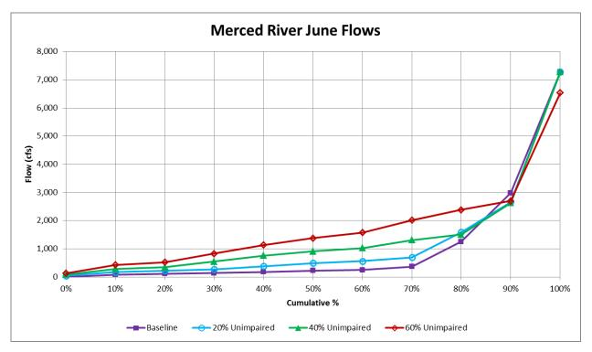
Figure F.1.4-1f. WSE-Simulated Cumulative Distributions of Merced River June Flows (cfs) at Stevinson for Baseline Conditions and 20%, 40%, 60% Unimpaired Flow (LSJR Alternatives 2–4)
