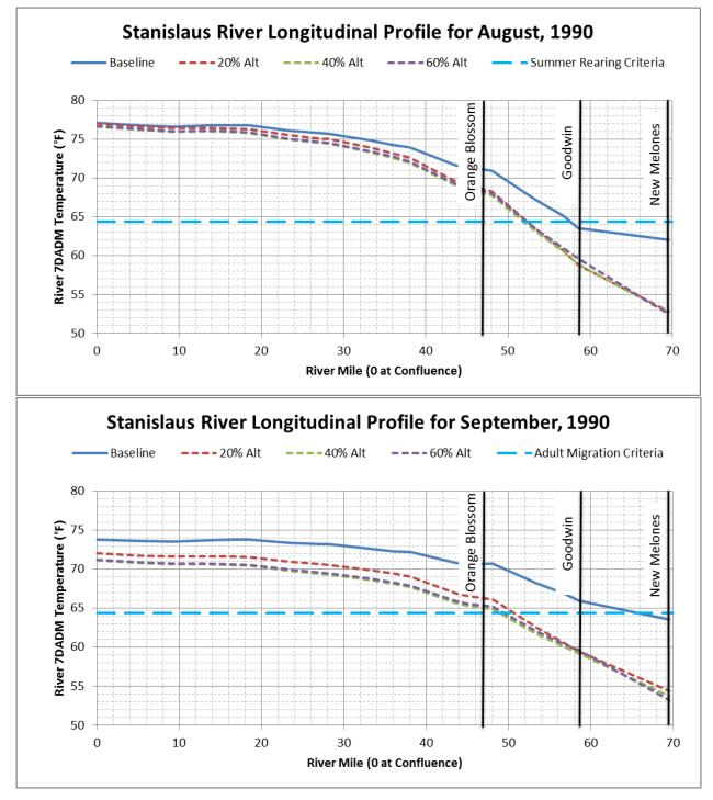
Figure F.1.6-25. Longitudinal Monthly Average 7DADM Temperature Results within the Stanislaus River for (a) August 1990 and (b) September 1990Error! Bookmark not defined.
