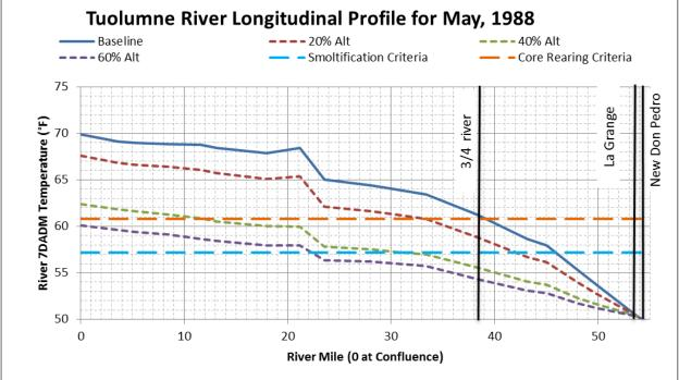
Figure F.1.6-35. Longitudinal Monthly Average 7DADM Temperature Results within the Tuolumne River for (a) April 1988 and (b) May 1988
