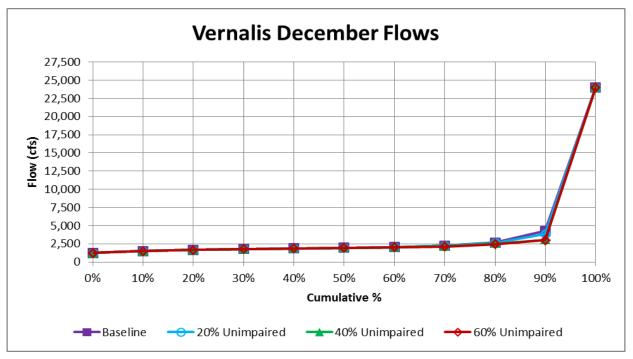
Figure F.1.4-4I. WSE-Simulated Cumulative Distributions of SJR at Vernalis December Flows (cfs) for Baseline Conditions and 20%, 40%, 60% Unimpaired Flow (LSJR Alternatives 2–4)
