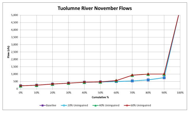
Figure F.1.4-2k. WSE-Simulated Cumulative Distributions of Tuolumne River November Flows (cfs) at Modesto for Baseline Conditions and 20%, 40%, 60% Unimpaired Flow (LSJR Alternatives 2–4)
