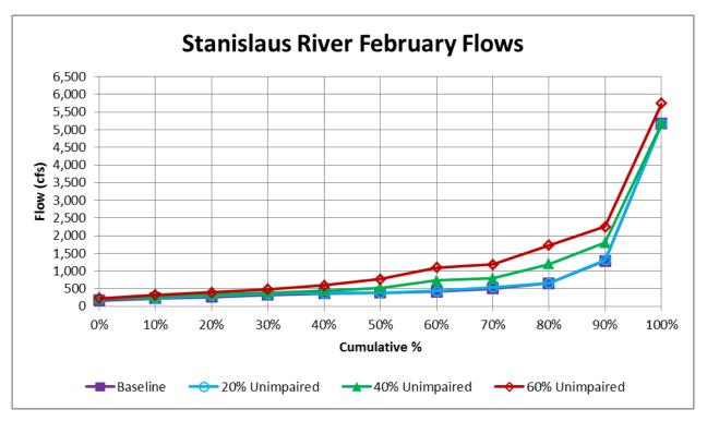
Figure F.1.4-3b. WSE-Simulated Cumulative Distributions of Stanislaus River February Flows (cfs) at Ripon for Baseline Conditions and 20%, 40%, 60% Unimpaired Flow (LSJR Alternatives 2–4)
