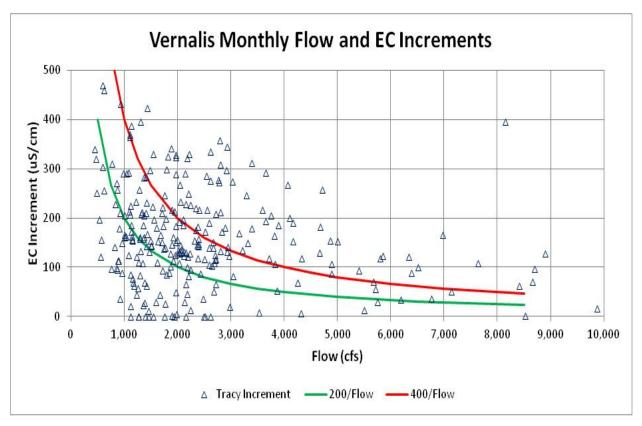
Figure F.1.5-2b. Historical Monthly EC Increments from Vernalis to Tracy Boulevard as a Function of Vernalis Flow (cfs) for Water Years 1985–2010)
