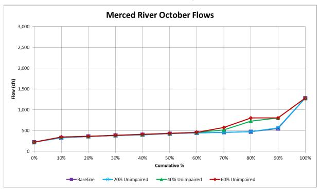
Figure F.1.4-1j. WSE-Simulated Cumulative Distributions of Merced River October Flows (cfs) at Stevinson for Baseline Conditions and 20%, 40%, 60% Unimpaired Flow (LSJR Alternatives 2–4)
