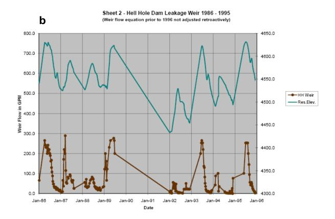
Figure E-2. Flows in Leakage Channel below Hell Hole Dam with Changes in Reservoir Water Surface Elevations 1978 to 1985 (a), Changes in Reservoir Water Surface Elevations 1986 to 1995 (b), Changes in Reservoir Water Surface Elevations 1996 to 2007 (c), and at Reservoir Elevations 4,580 and 4,540 feet (d) (continued).
