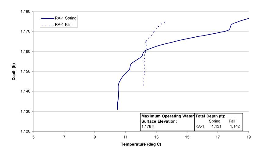
Figure C-1. Ralston Afterbay (RA-1) Temperature Profiles for the Spring and Fall Sampling Events.
