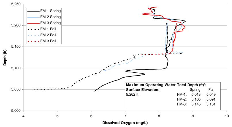
Figure C-6. French Meadows Reservoir (FMH-1, FM-2, FMH-3) Dissolved Oxygen Profiles for the Spring and Fall Sampling Events.
