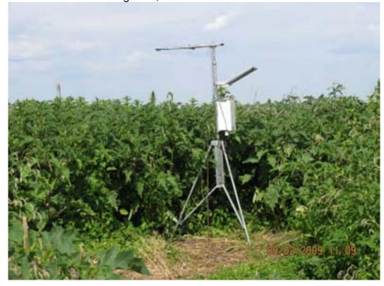
The sonic anemometer, installed with the rover, is completely surrounded by vegetation.
