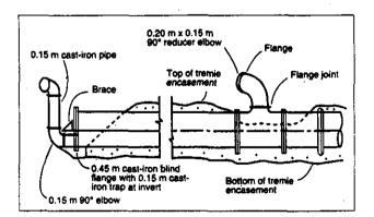
Figure 4-1. A Typical Diffuser Section [17]
