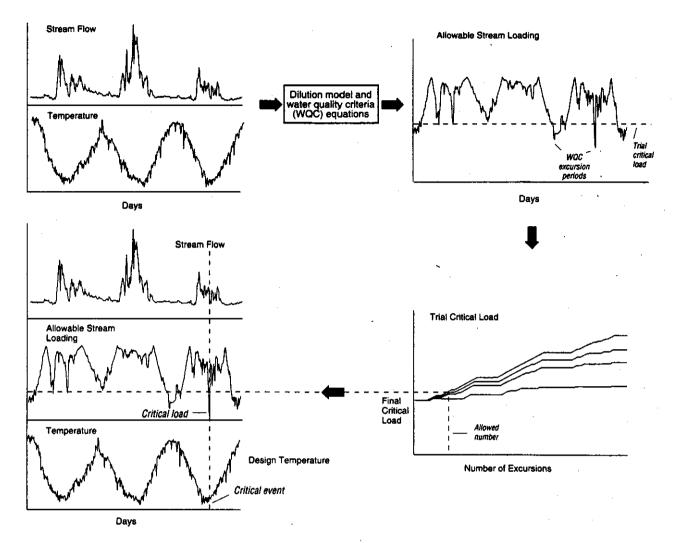
Figure 4-3. Computational Scheme for Deriving Design Conditions
