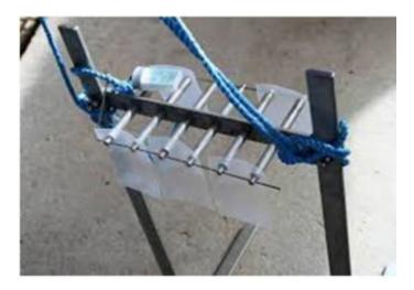
Figure 5. Micro-extraction devices
