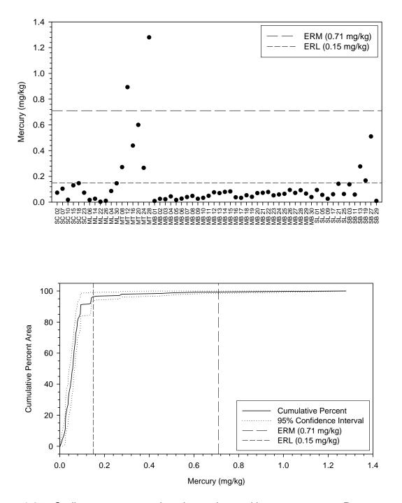
Figure 4-25. Sediment mercury values by station and by percent area. Percent areas were calculated by the cumulative distribution function (CDF). Dashed lines represent Effects Range Low (ERL) and Effects Range Median (ERM) guideline values associated with potential toxic biological events (Long et al. 1995). SC=Santa Cruz, ML=Moss Landing, MB=Morro Bay, SL=Port San Luis, SB=Santa Barbara.
