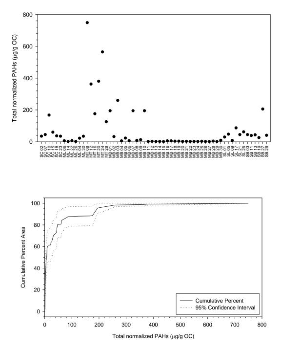
Figure 4-37. Sediment total normalized PAH values by station and by percent area. Values were normalized to total organic carbon (TOC) content. Percent areas were calculated by the cumulative distribution function (CDF). No value exceeded the Swartz (1999) consensus guideline of 1,800  $\mu$ g/g OC. SC=Santa Cruz, ML=Moss Landing, MB=Morro Bay, SL=Port San Luis, SB=Santa Barbara.
