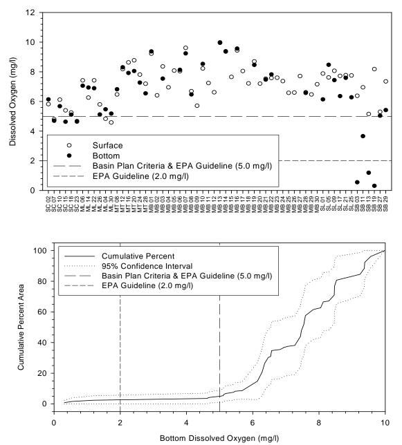
Figure 4-4. Water dissolved oxygen values by station and by percent area. Stations indicate surface and, where applicable, bottom dissolved oxygen. Percent areas were calculated by the cumulative distribution function (CDF). Assessment values represent Central Coast RWQCB Basin Plan criteria (5.0 mg/l; RWQCBCC 1994) and US EPA National Coastal Condition Assessment guidelines (2.0 and 5.0 mg/l; USEPA 2004). SC=Santa Cruz, ML=Moss Landing, MB=Morro Bay, SL=Port San Luis, SB=Santa Barbara.
