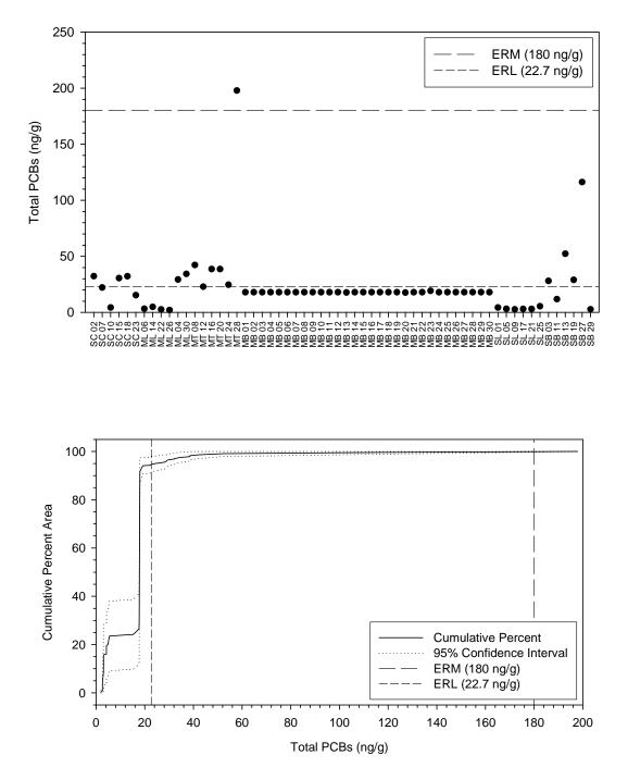
Figure 4-33. Sediment total PCB values by station and by percent area. Percent areas were calculated by the cumulative distribution function (CDF). Dashed lines represent Effects Range Low (ERL) and Effects Range Median (ERM) guideline values associated with potential toxic biological events (Long et al. 1995). SC=Santa Cruz, ML=Moss Landing, MB=Morro Bay, SL=Port San Luis, SB=Santa Barbara.
