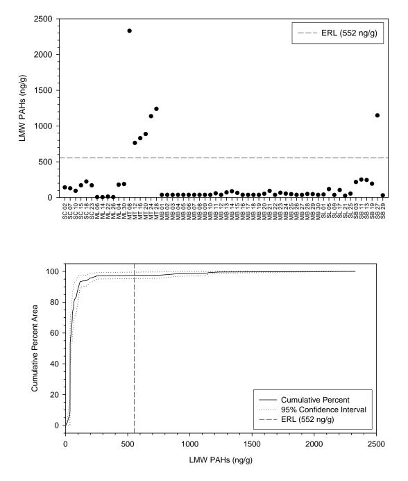
Figure 4-34. Sediment low molecular weight (LMW) PAH values by station and by percent area. Percent areas were calculated by the cumulative distribution function (CDF). Dashed line represents the Effects Range Low (ERL) guideline value associated with potential toxic biological events (Long et al. 1995). SC=Santa Cruz, ML=Moss Landing, MB=Morro Bay, SL=Port San Luis, SB=Santa Barbara.
