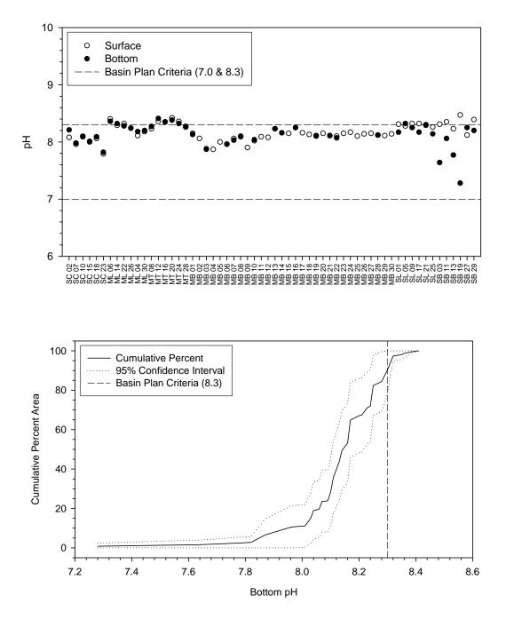
Figure 4-3. Water pH values by station and by percent area. Stations indicate surface and, where applicable, bottom pH. Percent areas were calculated by the cumulative distribution function (CDF). Criteria values represent Central Coast RWQCB Basin Plan values (RWQCBCC 1994). SC=Santa Cruz, ML=Moss Landing, MB=Morro Bay, SL=Port San Luis, SB=Santa Barbara.
