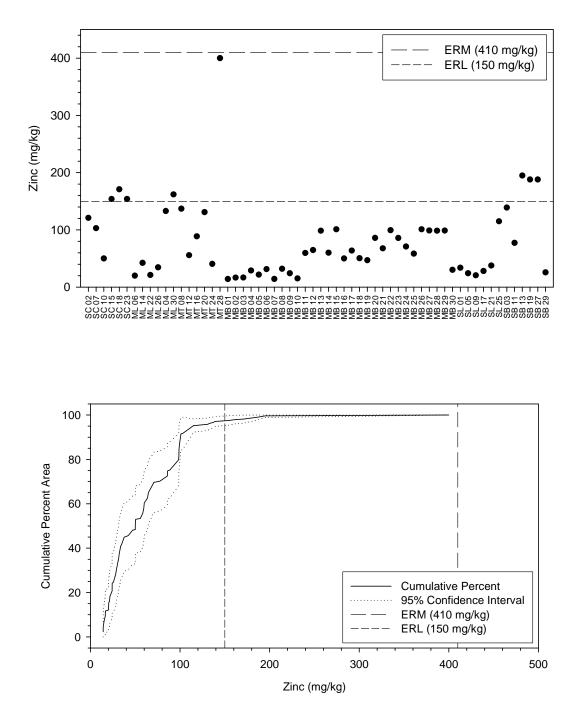
Figure 4-29. Sediment zinc values by station and by percent area. Percent areas were calculated by the cumulative distribution function (CDF). Dashed lines represent Effects Range Low (ERL) and Effects Range Median (ERM) guideline values associated with potential toxic biological events (Long et al. 1995). SC=Santa Cruz, ML=Moss Landing, MB=Morro Bay, SL=Port San Luis, SB=Santa Barbara.
