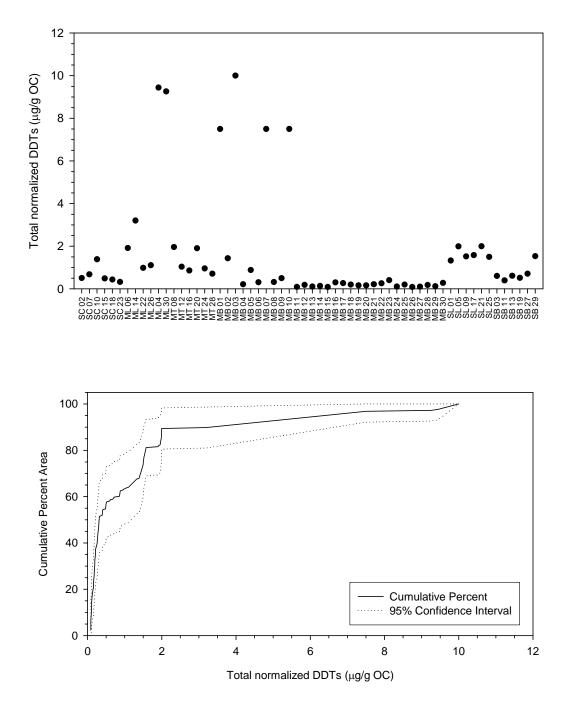
Figure 4-32. Sediment total normalized DDTs values by station and by percent area. Values were normalized to total organic carbon (TOC) content. Percent areas were calculated by the cumulative distribution function (CDF). No value exceeded the consensus guideline of 100  $\mu$ g/g OC (Swartz et al. 1994). SC=Santa Cruz, ML=Moss Landing, MB=Morro Bay, SL=Port San Luis, SB=Santa Barbara.
