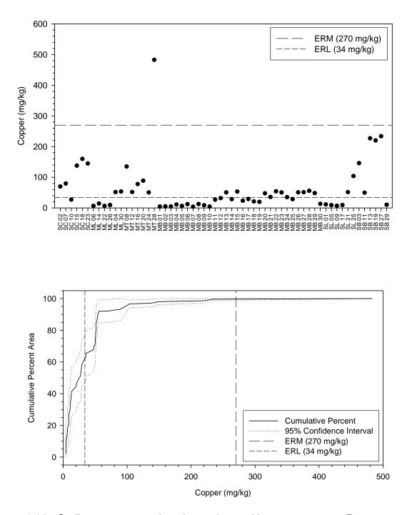
Figure 4-22. Sediment copper values by station and by percent area. Percent areas were calculated by the cumulative distribution function (CDF). Dashed lines represent Effects Range Low (ERL) and Effects Range Median (ERM) guideline values associated with potential toxic biological events (Long et al. 1995). SC=Santa Cruz, ML=Moss Landing, MB=Morro Bay, SL=Port San Luis, SB=Santa Barbara.
