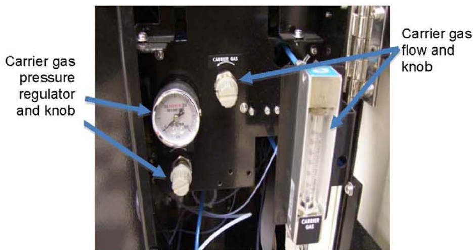
Figure 3. Setting the carrier gas pressure and flow.
