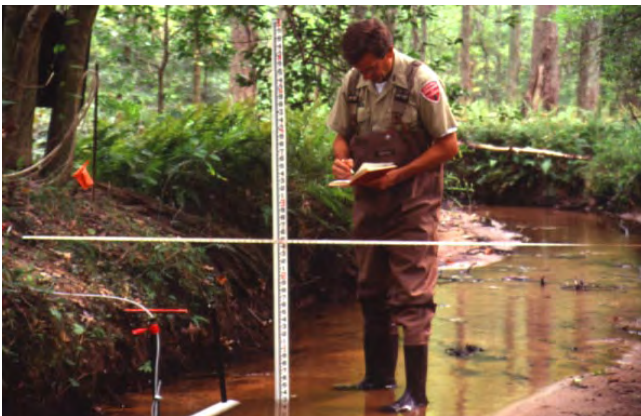
Figure 11: Measuring bankfull stage
