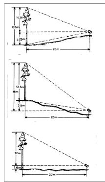
Figure 5. Determining height
