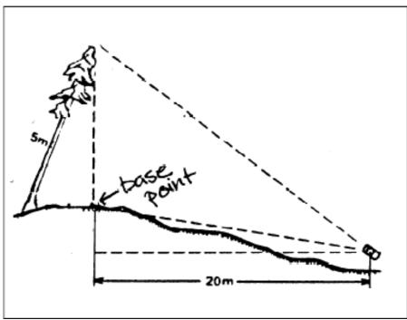
Figure 6. Where tree is leaning or misshapen, it is critical to measure from directly below the highest visible point of the tree, rather than from the base of the tree itself.
