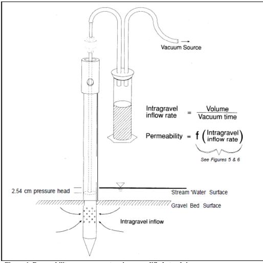
Figure 1. Permeability measurements using a modified standpipe.
