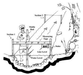
Figure 4. Taglines marking ends of stream segment used for float measurement
