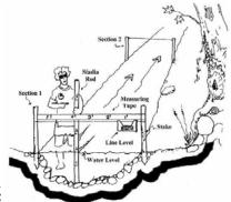
so it can be recorded on the Stream Flow Field Sheet. Please read the section on How to Read the Stadia Rod.
