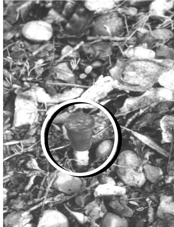
Figure 2. Rebar benchmark with plastic cap.
