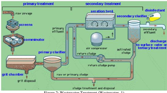
Figure 2: Wastewater Treatment (Wastewater, 1)
