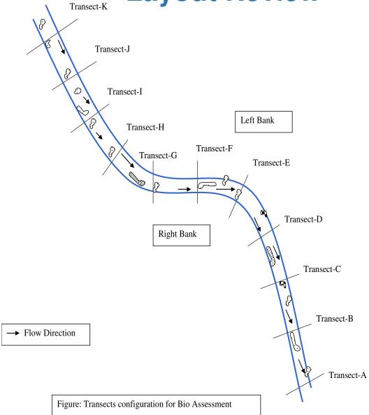
Figure 1. Reach layout geometry for physical habitat and biological sampling showing positions of 11 main transects (A – K) The area highlighted in the figure is expanded in Figure 2. Note: reach length = 150 m for streams 10 m average wetted width and reach length = 250 m for streams > 10 m average wetted width.
