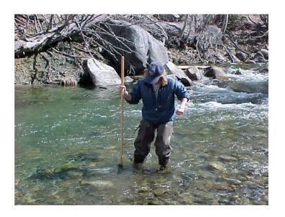
RWB -Step 5. Vigorously kick the remaining finer substrate within the quadrat with your feet while dragging the net repeatedly through the disturbed area just above the bottom. Keep moving the net all the time so that the organisms trapped in the net will not escape.
