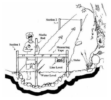
NBO-Step 4. Place a neutrally buoyant object (e.g., orange, rubber ball, heavy piece of wood, etc.) in the water upstream of the discharge reach and record the length of time in seconds that it takes for the object to pass between the upstream and downstream boundaries of the reach. Repeat this timed float three times.
