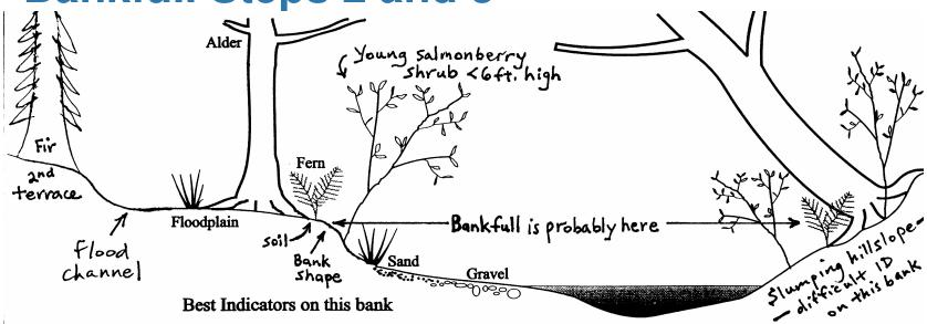
Step 2. Stretch a tape from bank to bank at the bankfull position. Measure the width of the bankfull channel from bank to bank at bankfull height and perpendicular to the direction of stream flow.
