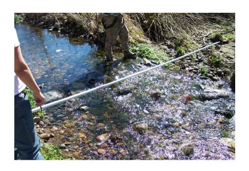
Step 3. Determine if the average wetted width is greater or less than 10 m. If average wetted width is less than 10 m use a 150 m reach length If average wetted width > 10 m then use a 250 m reach length.
