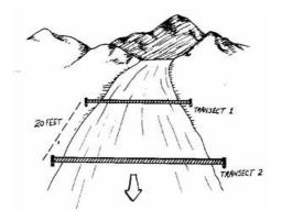
NBO-Step 2. The cross sectional area is estimated in a manner that is similar but less precise than that used in the velocity area method. Measure the cross sectional area in one to three places in the section designated for the discharge measurement (three evenly spaced cross sections are preferred, but one may be used if the cross section through the reach is very uniform). Record the width once for each cross section and measure depth at five equally-spaced positions along each transect.
