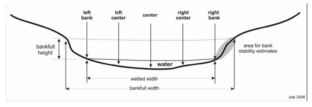
Bankfull Width and Depth~ The bankfull channel is the zone of maximum water inundation in a normal flow year (one to two year flood events). Since most channel formation processes are believed to act when flows are within this zone (Mount 1995), bankfull dimensions provide a valuable indication of relative size of the waterbody.
