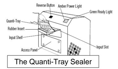
2 Place the Quanti-Tray/Inset onto the input shelf and feed it into the sealer.
