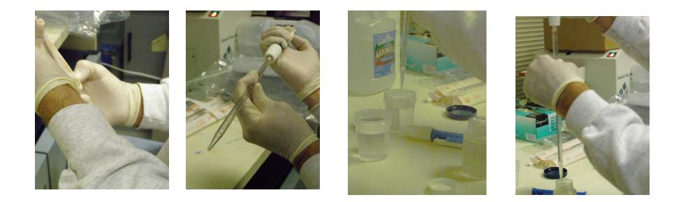
Prepare a sterile pipette and take some of the sample water (10ml or 1ml depending on Dilution rate desired).
