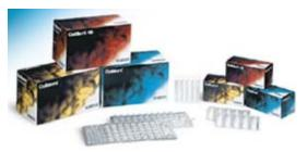
Colilert: measures coliform bacteria for freshwater Colilert-18 Measures coliform bacteria for marine waters Enterolert: measures enterococcus bacteria
