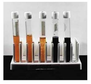
The **multiple-tube fermentation** method involves adding specified quantities of the sample to tubes containing a nutrient broth, incubating the tubes at a specified temperature for a specified time period, and then looking for the development of gas and/or turbidity that the bacteria produce. The presence or absence of gas in each tube is used to calculate an index known as the **Most Probable Number** (MPN).
