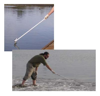
Sediment not effected. Gloves worn. Equipment decontaminated. Sampling vessels are sterile. Samples obtained subsurface.
