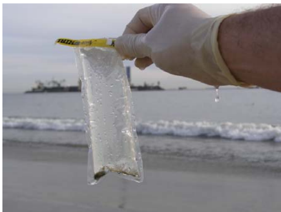
Bad- No air space (For FIB Samples)
