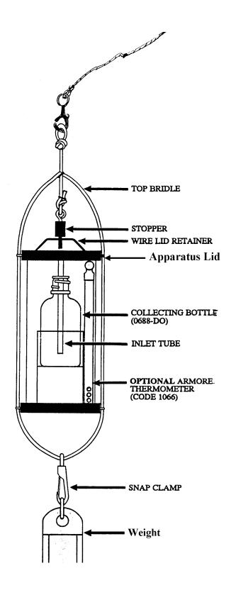
Figure 1: Schematic representation of the LaMotte sampling apparatus
