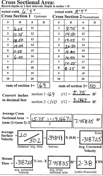
Figure 3-38: Stream Flow Field Sheet
