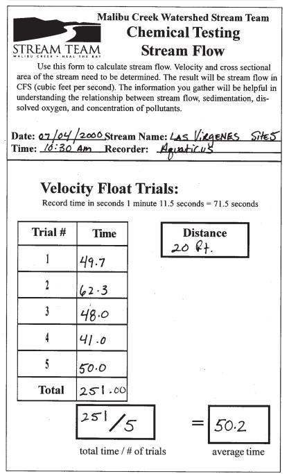
Figure 3-39: Stream Flow Velocity Float Trials Field Sheet
