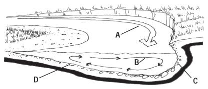
Figure 2-11:Erosion and deposition along stream curves: A) path of current around curve, B) circulatory current in water flowing around curve, C) area of erosion and D) area of deposition (from figure 28, Leopold"Water, Rivers and Creeks" 1997)
