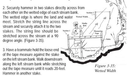
4. Repeat step 2 on the right stream bank and attach the string line on the downstream stakes. You should have 2 sets of stakes and string lines stretched across the stream, 20 feet apart (Figure 3-35).
