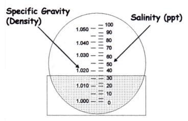
Figure 3-27: Reading the salt refractometer scale
