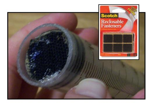
Obtain some white scrubbing pad material (make sure it is not pigmented so it will not end up interfering with eventual chlorophyll *a* analysis of the samples collected.) Cut a supply of circles to fit the size of the plunger.
