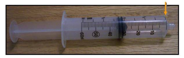
Firmly affix the rubber end to the plastic plunger by removing the rubber tip, applying glue to the "naked" end of the plunger, and *replacing the rubber cap*. Allow glue to cure. Then cut the conical part off the plunger tip so that only a flat surface of rubber remains.
