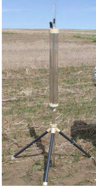
Figure C-3: Guelph Permeameter for Shallow Borehole Permeability
