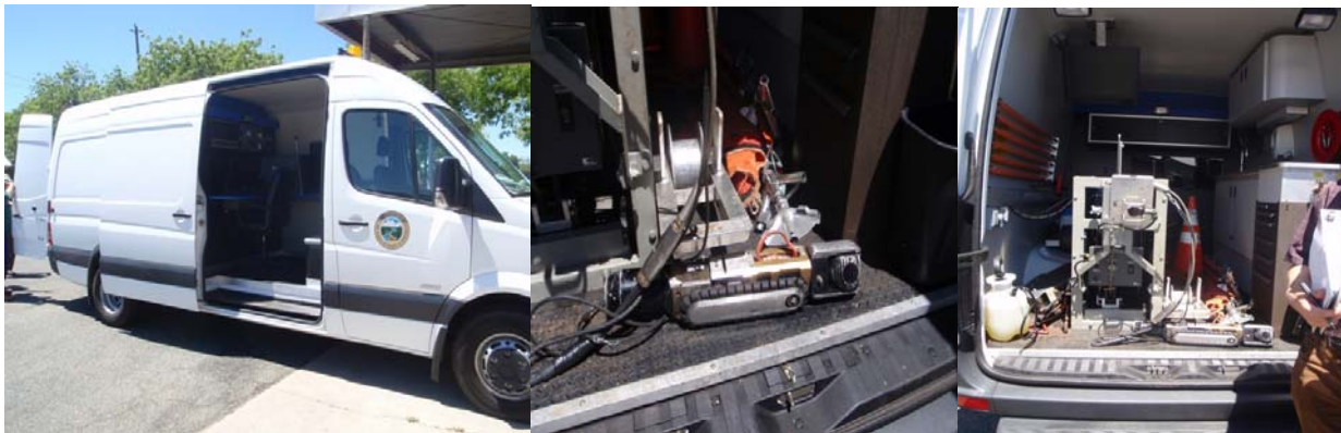
Photos 1-3: City maintenance shop [CCTV truck and associated equipment]
