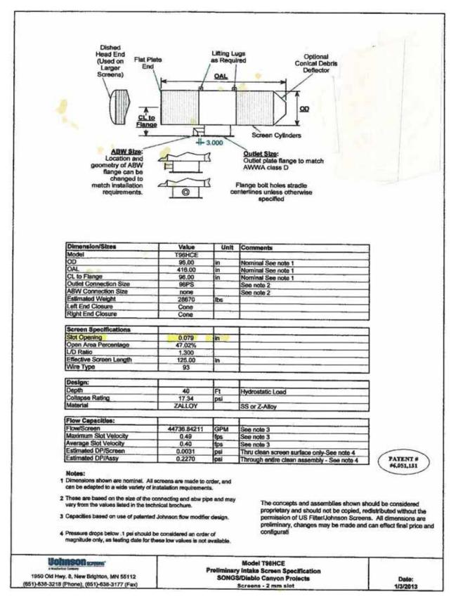
Figure 4.2-21. DCPP Preliminary Intake Screen Specifications (2-mm Slots)
