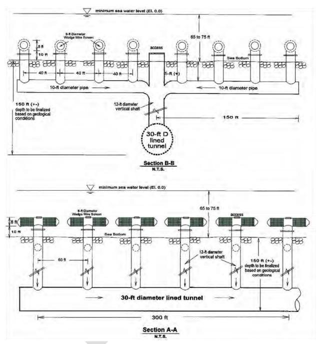
Figure 4.2-9. DCPP 2-mm-Slot Wedge Wire Screen Intake System (Sectional Views)
