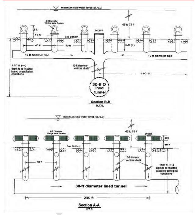
Figure 4.2-7. DCPP 6-mm-Slot Wedge Wire Screen Intake System (Sectional Views)
