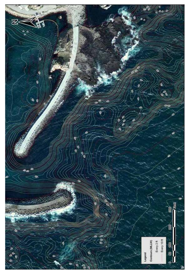
Figure 4.2-2. DCPP Bathymetry Map (Contour elevations = feet below MLLW)
