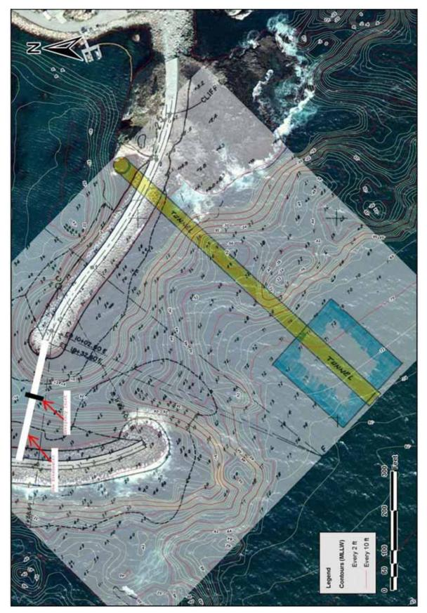
Figure 4.2-3. DCPP Bathymetry/Tunnel for 6-mm-Slot Screen Layout (Contour elevations = feet below MLLW)
