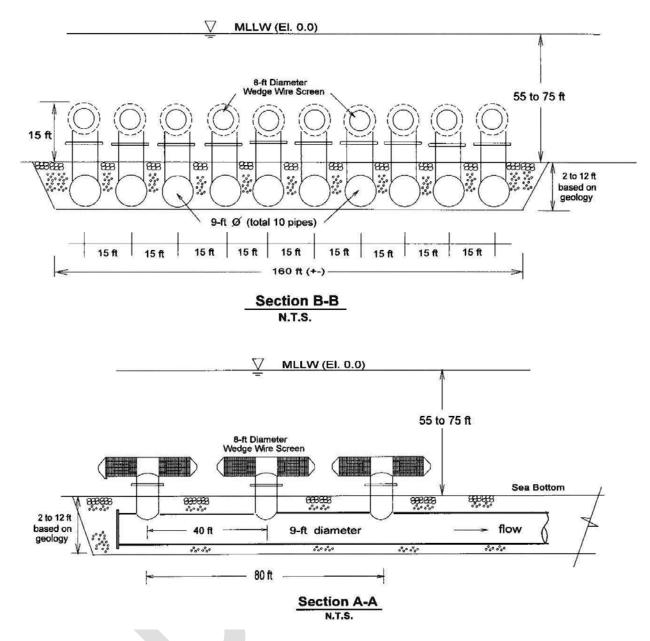
Figure 4.2-15. DCPP 6-mm-Slot Wedge Wire Screen Intake Assembly (Sectional Views)
