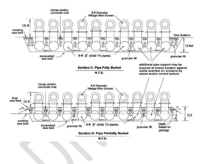
Figure 4.2-18. DCPP Potential Buried Pipe Trench Scenarios (Based on Seabed Geology)
