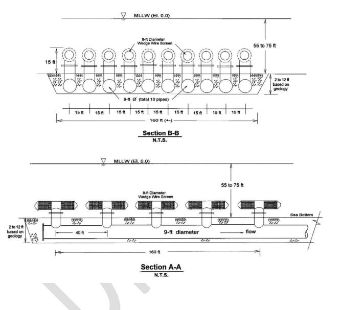
Figure 4.2-17. DCPP 2-mm-Slot Wedge Wire Screen Intake Assembly (Sectional Views)
