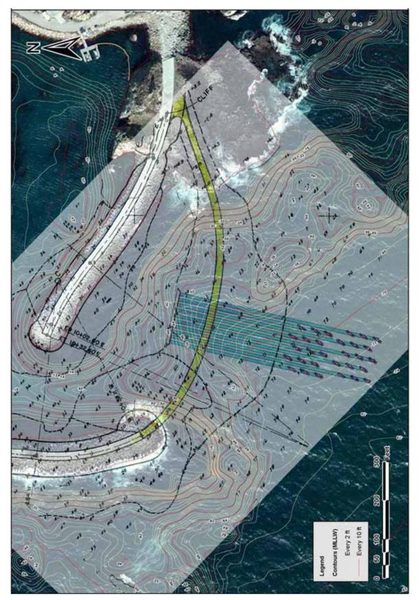
Figure 4.2-11. DCPP Bathymetry/Buried Pipe Layout with 6-mm-Slot Screens (Contour elevations = feet below MLLW)
